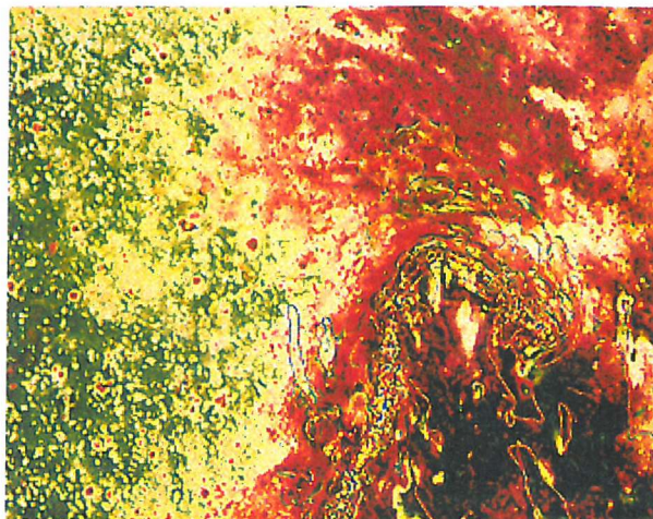
Figure 4.10 : Glassy texture exhibited by CBO4O2CP at 25°C (magnification x100).
