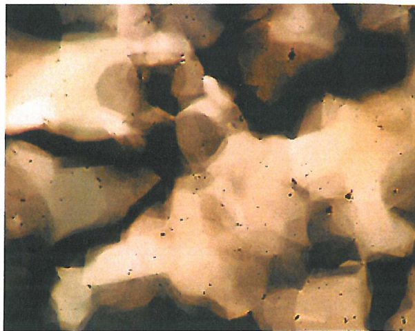
Figure 4.19 : The characteristic platelet texture exhibited by the E phase of CTO11O2CP on cooling from the homeotropic SmA/B phase at 120°C (magnification x100).
