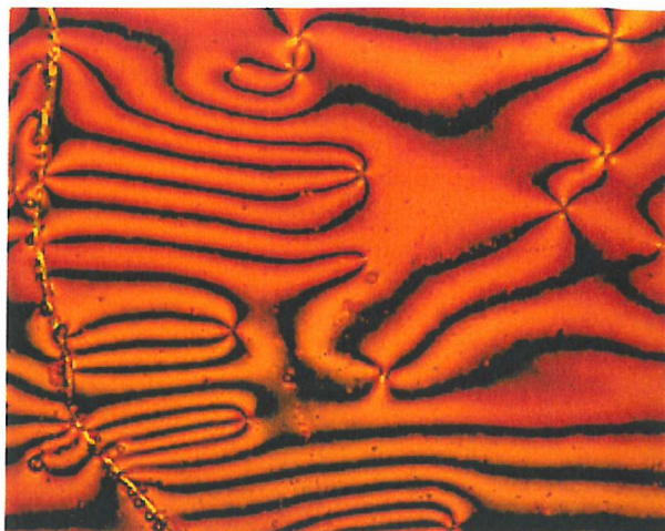
Figure 2.16 : The optical texture exhibited by the nematic phase of an equimolar mixture of C9SD and TNF on cooling at 150°C (magnification x100).
