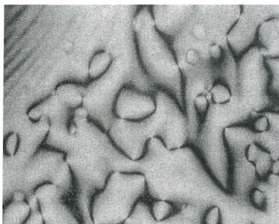
Figure 5.5 : The schlieren texture consisting of only two-point brushes that has been suggested will form for a thermotropic biaxial nematic phase.
