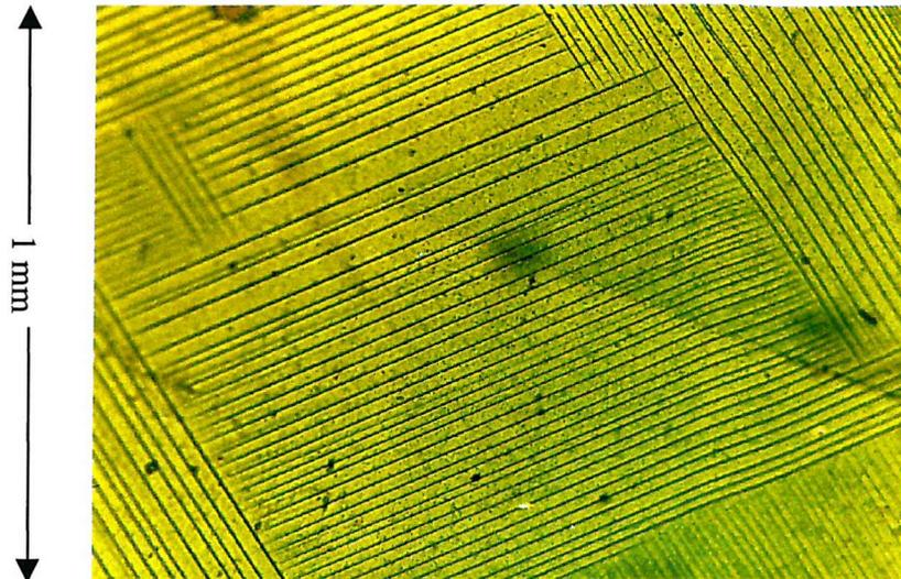
Fig. 3.8. The surface of a twinned  $\text{YBa}_2\text{Cu}_3\text{O}_{7-\delta}$  single crystal as seen using a polarized light microscope. The straight black lines represent the two sets of twin planes formed in the directions  $[110]$  and  $[1-10]$ .
