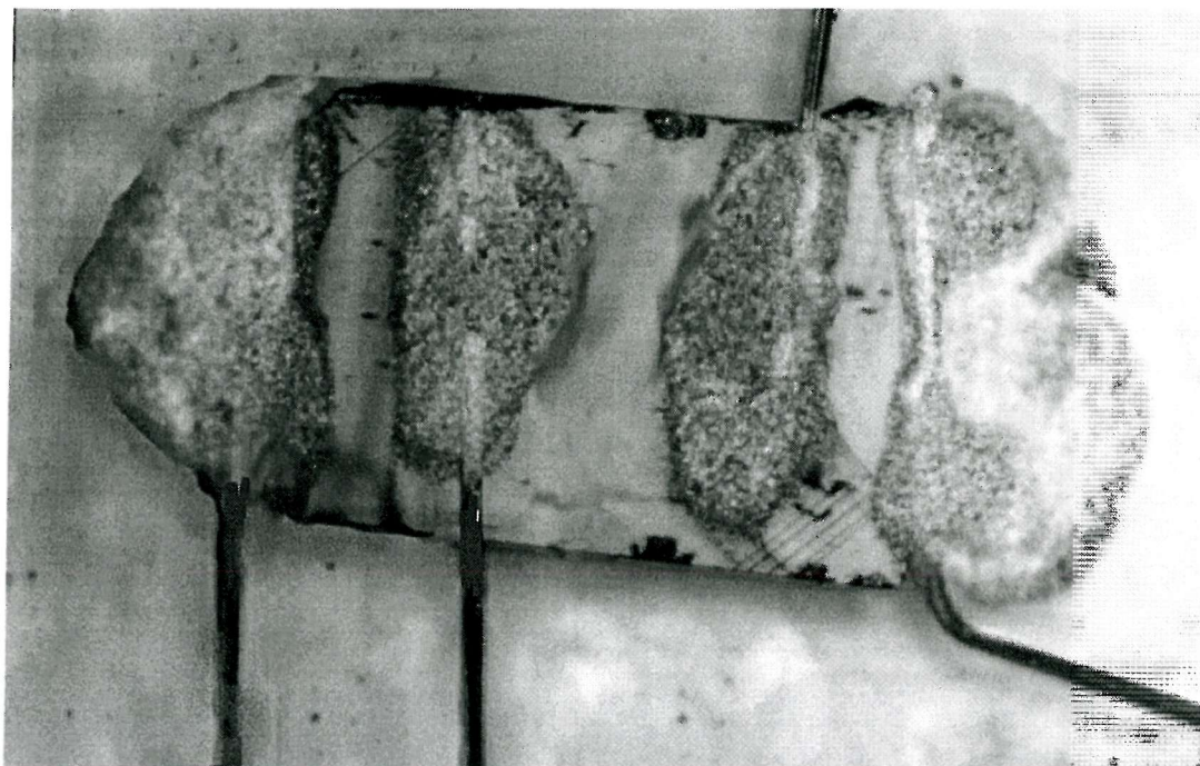
Fig. 2.5 Typical four point contact-configuration, attached to a partially detwinned \text{YBa}_2\text{Cu}_3\text{O}_{7-\delta} single crystal as photographed under polarised light microscopy. Notice the region of residual twin-planes in the bottom right-hand corner of the sample.
