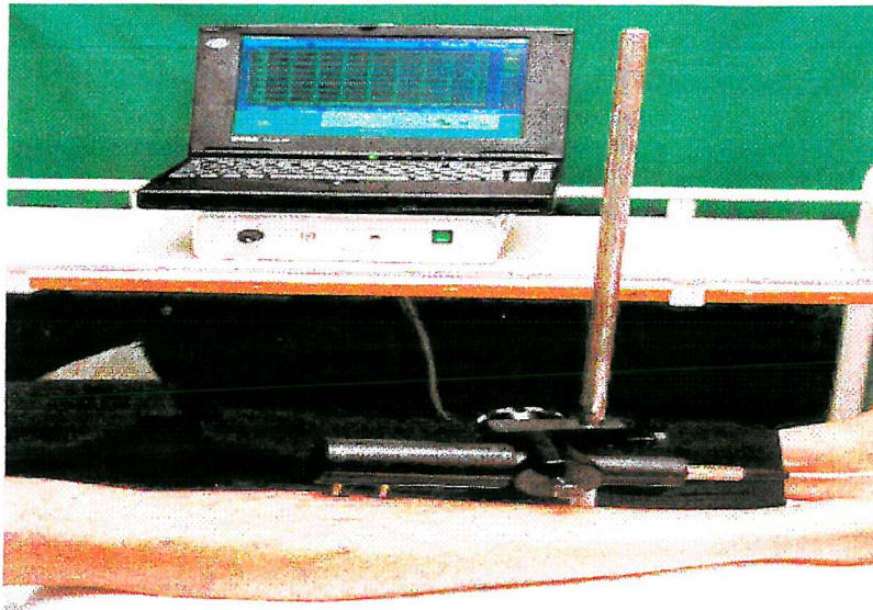
Figure 3.6 The extensometer and data acquisition system.
