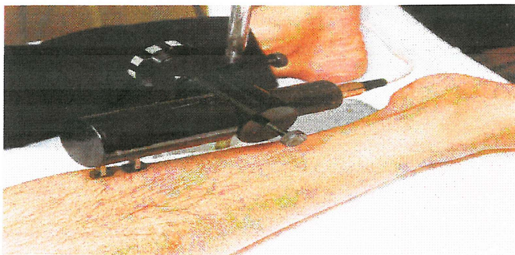
Figure 3.5 Uniaxial extensibility/relaxation measurement on the medial aspect of the leg. The extensometer feet were glued to the skin using cyanoacrylate adhesive, without applying pressure or suction.
