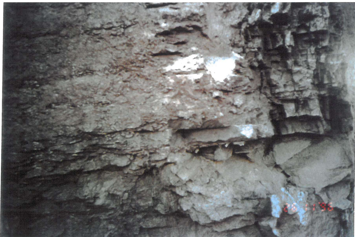
Figure 3.5. Typical jointing for the area
