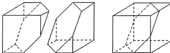
Figure 5.1 Hexagonal bisection of a cube.
