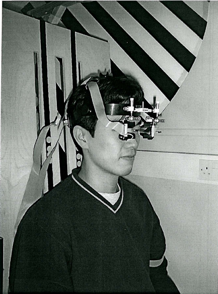
Figure 3.13. A subject shown wearing the IRIS eye position sensors.
