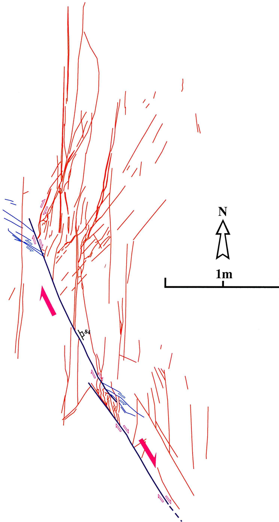
Fig. 3.6. A strike-slip fault (F23) showing tip cracks on both sides of the main fault tip. Although tip cracks associated with right-lateral movement are predominant, minor tip cracks associated with left-lateral reactivation are evident.
