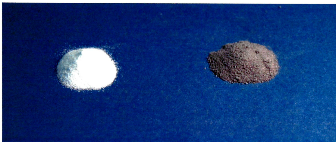
Figure 4.6: Picture of the beads, en masse, showing traditional (left) and the magnetic beads (right).
