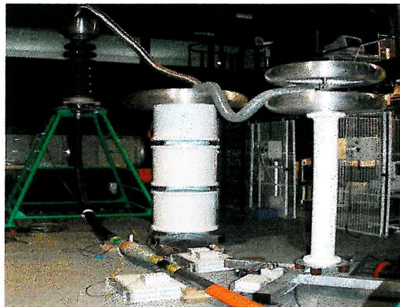
Figure 7.1 Schematic diagram for the 132 kV cable/joint PD test arrangement
