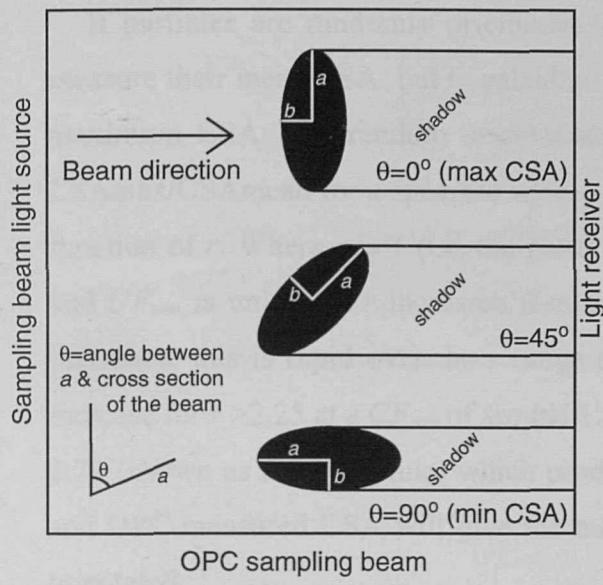
**Figure 3.2.2.ii** Graph showing the CSA of a spheroid from Eq 3.2.3 at various angles (where  $a = 800 \mu\text{m}$ ,  $b = 294 \mu\text{m}$ )
