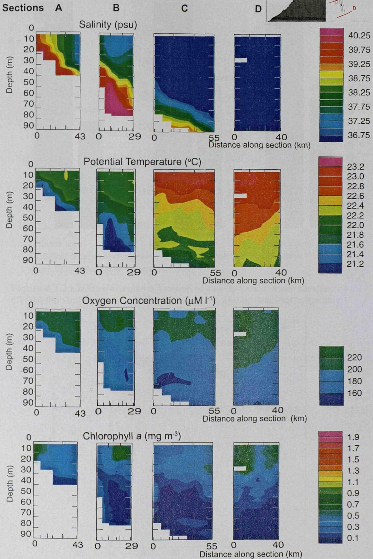
**Figure 4.1.1.iv** Full depth CTD data from Line D: profiles of salinity, temperature and dissolved oxygen. This is the same section as in Fig 4.1.1.iii, but contoured to the full depth of the sea floor
