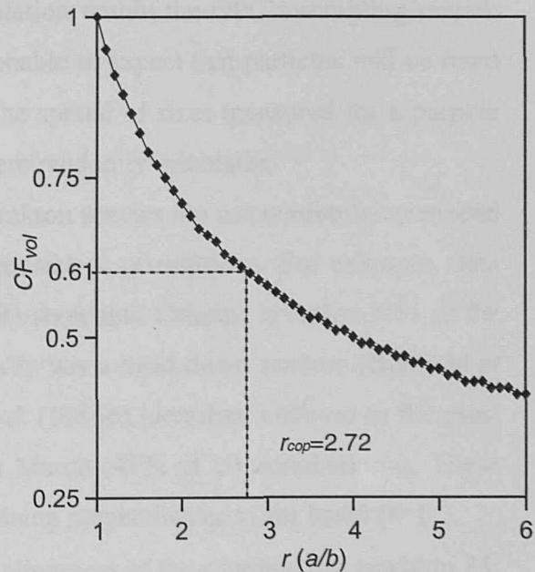
Using the average spheroid ( $r_{cop} = 2.72:1$ ,  $a = 800 \mu\text{m}$ ,  $b = 294 \mu\text{m}$ ) the mean  $CSA_{opc}$  of randomly orientated particles is  $0.61 \text{ mm}^2$ , which is 82% of the maximum CSA (shown as dotted line on **Fig 3.2.2.ii**).
