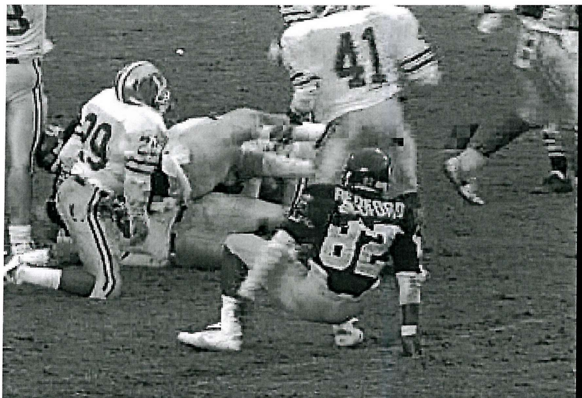
Figure 2.27: Frame 79 of "Football" sequence, which illustrates the visual effects of minor decoding errors at a BER of 2 \cdot 10^{-4} after convolutional decoding. The PSNR degradation observed is approximately 2 dB. The sequence was coded using a rate 7/8 convolutional code and transmitted employing QPSK modulation.
