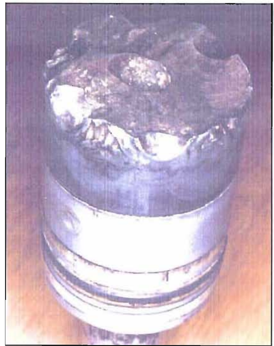
Figure 1-2 Sand Erosion of the Plug of a 3" Control Choke
