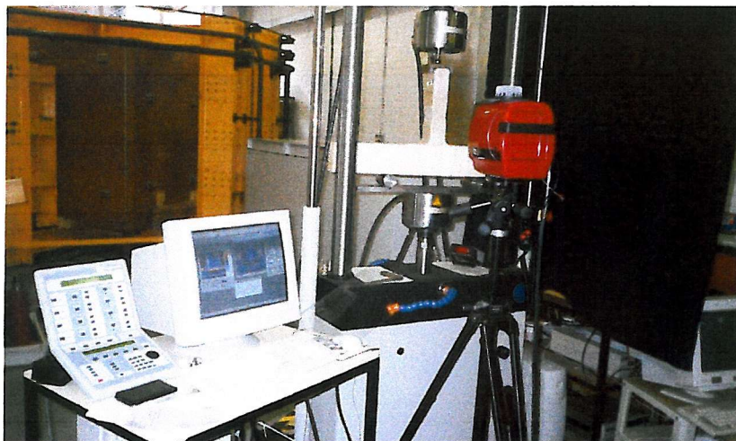
Figure 11.3: DeltaTherm test set-up for aged joint work (note chamber within the yellow steelwork of FORTReSS in the background)
