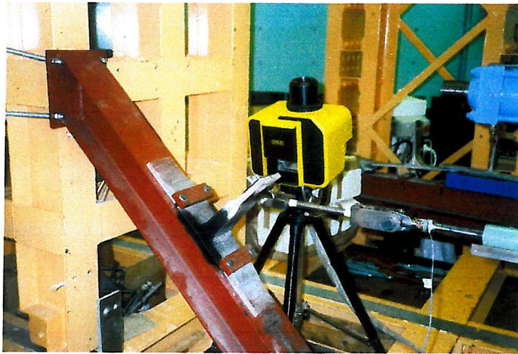
Figure 6.3: SPATE Equipment Scanning Single Skin Tee Joint Under 45° Pull-off Load in FORTReSS
