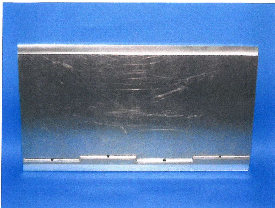
Figure 5-3. Picture showing the condensate collection gutters, cut into the condenser side wall.
