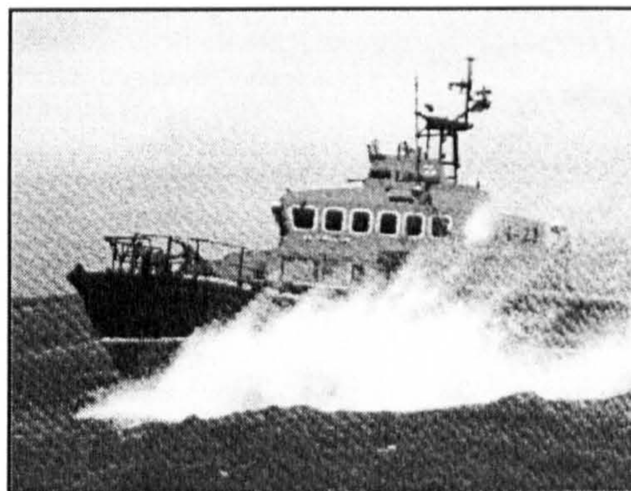
Figure 1.1: R.N.L.I. Trent Class lifeboat (the hull is made of glass/kevlar epoxy skins and a closed cell polymer foam core).
