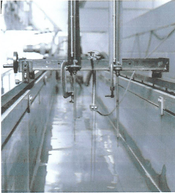
Figure 5.4 Two point gauges and surface penetrating wave probe fixed to moveable trolley.
