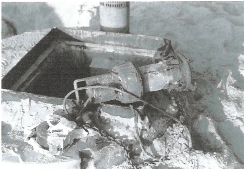
Figure 3.36: Corroded pump (June 1999)
