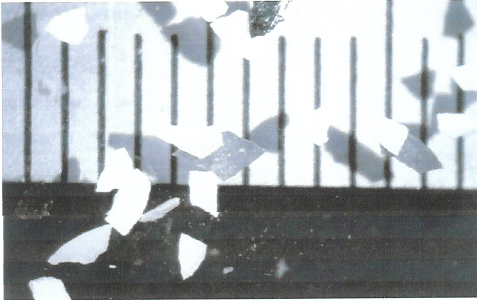
Figure 5.11a: Platy particles present in the Bakelite sediment sample (millimetre scale is shown behind the sample)
