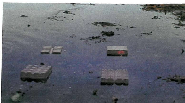
Plate (5.1): Each of the four block types placed into the intertidal zone of Camas Rubha na Liathaig.
