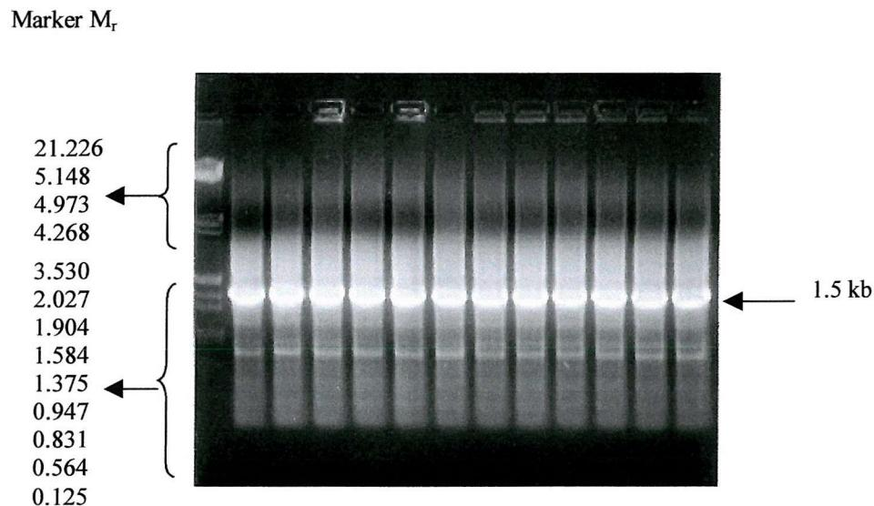
**Figure 4.7 PCR 2 to generate the native ALAS using T388S DNA as a template with PCR primers containing *Bam*HI and *Eco*RI sites**
