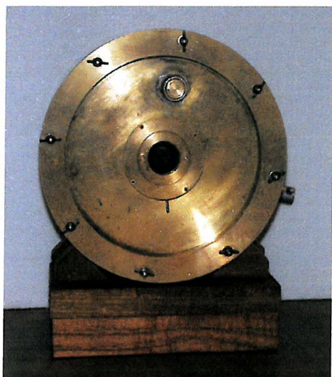
Figure 3.14 Plaque sample holder for the LIPP system
