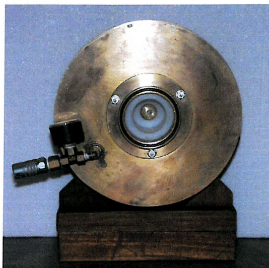
Figure 3.14 Plaque sample holder for the LIPP system
