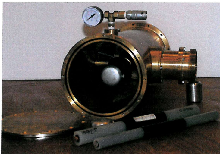
Figure 3.15 Cable sample holder for the LIPP system
