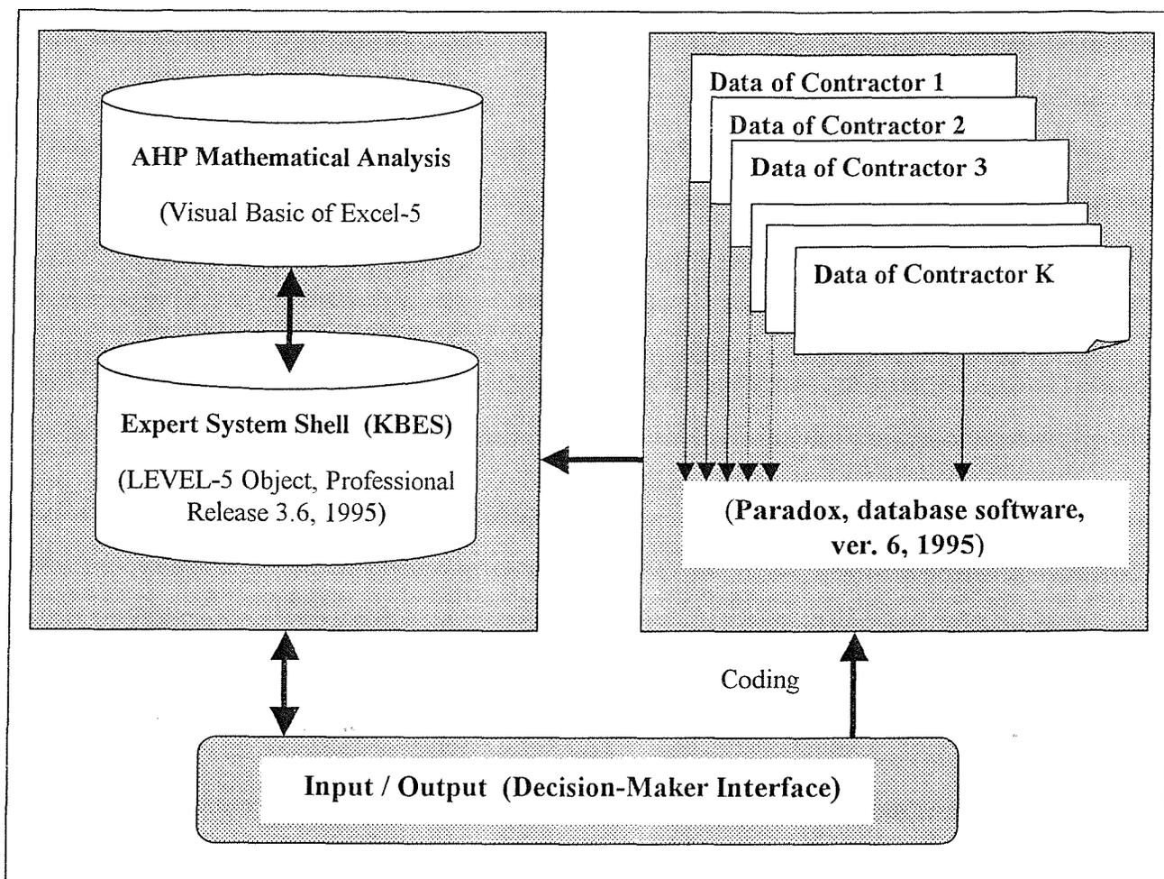
**Figure 7.3: The Construction of the KBES for Contractor Selection System.**
