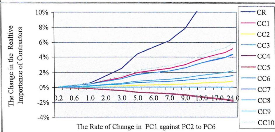
Figure 8.6.d: The Change in the Relative Importance of Contractors due to the Change in the Proj. Cost (PC1) vs (PC2) - (PC6) [Case-2]
