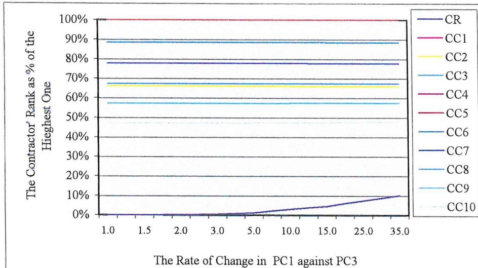
Figure 8.3.a: The Change in the Contractors' Rank due to the Change in the Proj. Cost (PC1) vs Proj. Quality (PC3) [Case-1]
