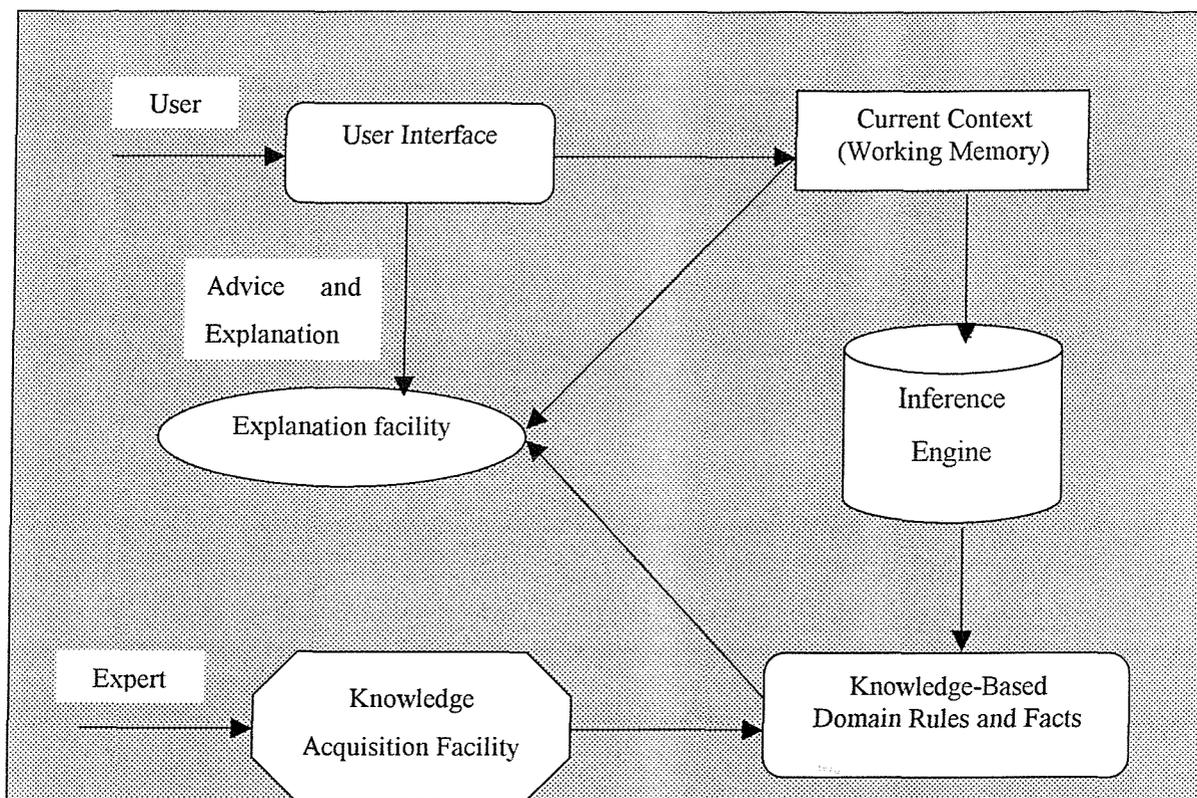
**Figure 6.4: The Components of a more Elaborate Knowledge-Based Expert System [KBES] (Maher, 1987)**
