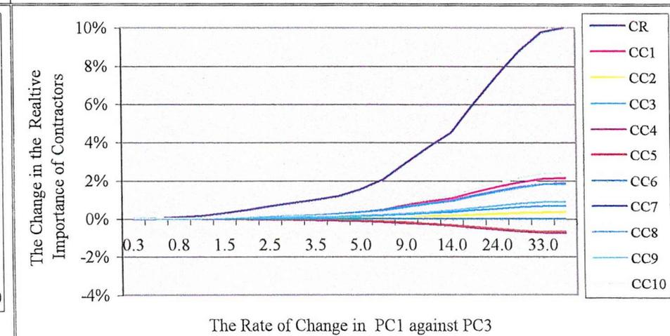
Figure 8.3.d: The Change in the Contractors Rank due to the Change in the Proj. Cost (PC1) vs Proj. Quality (PC3) [Case2]
