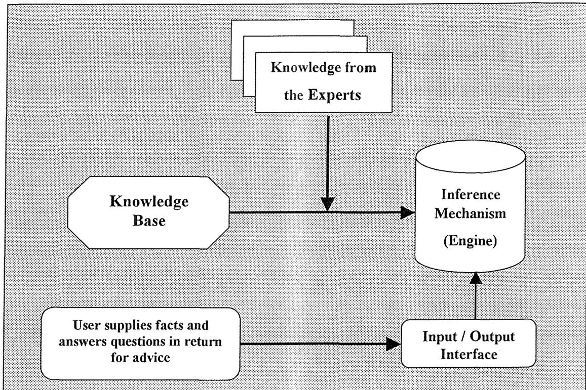
**Figure 6.3: The Architecture of a Typical KBES (Hart, 1986)**
