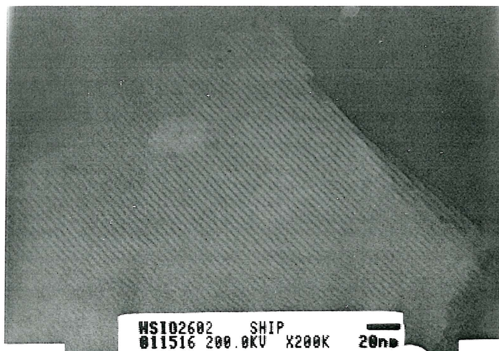
Figure 5.1 :- TEM micrograph showing the equidistant parallel lines arising from the mesoporous structure of \text{H}_1\text{SiO}_2 modified with \text{CH}_3\text{SO}_3\text{H} .
