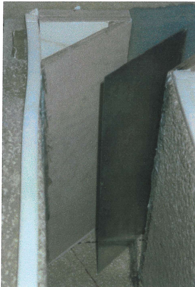
Figure 7.16 – Photograph of duct termination used to experimentally test the ‘horn’ hypothesis
