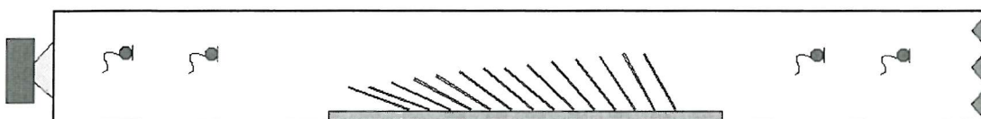
Figure 6.33 – Scale diagram of gradual angle change experimental set-up
