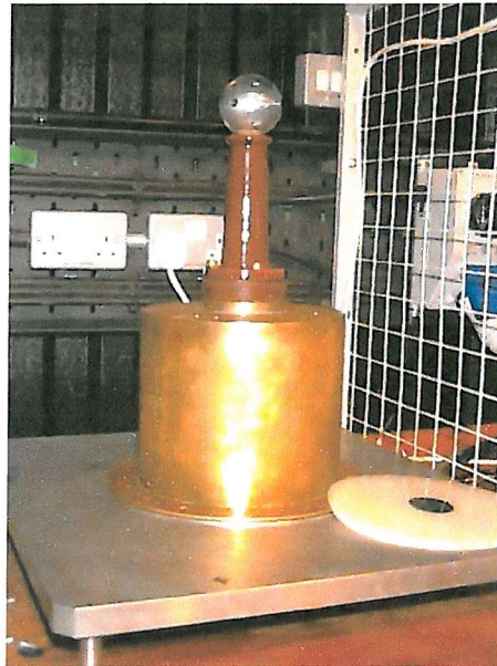
Figure 8.1 Photograph of the PEA electrodes system for the thick plaque sample
