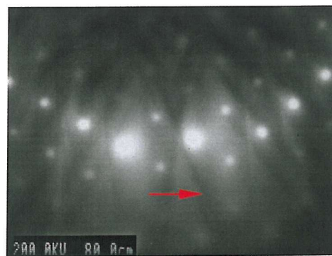
Figure 6.18. Bright-field XTEM micrographs of the linear-graded heterostructure of the first set, 775, showing the same pileup of TDs imaged in different two-beam conditions and the corresponding diffraction patterns: (a) the main beam condition; (b) 00\bar{2} ; (c) 1\bar{1}\bar{1} ; (d) \bar{1}11 ; (e) \bar{2}20 ; (f) 2\bar{2}0 . The fact that the TDs are visible in all two-beam conditions indicates their mixed type.
