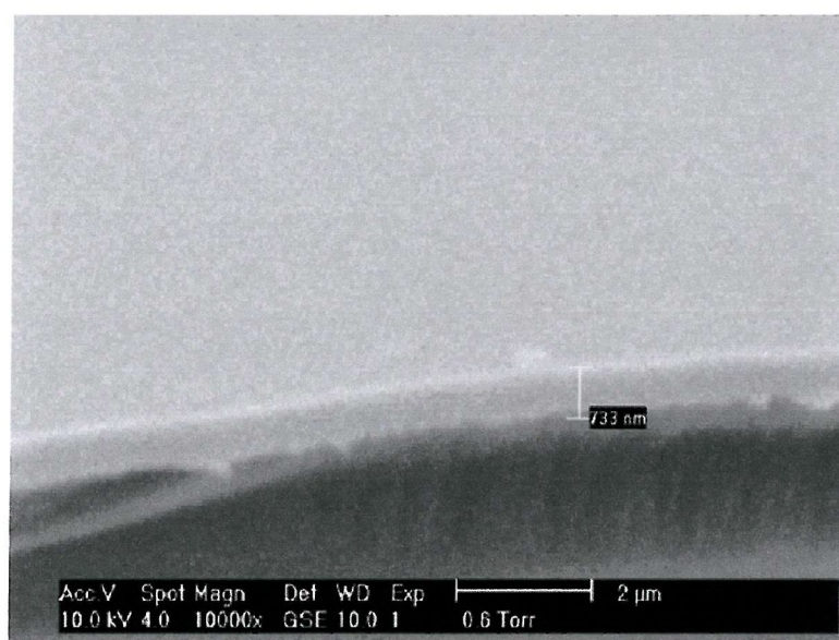
Figure 4.9: SEM image of the polymer film containing PC groups after hydration.
