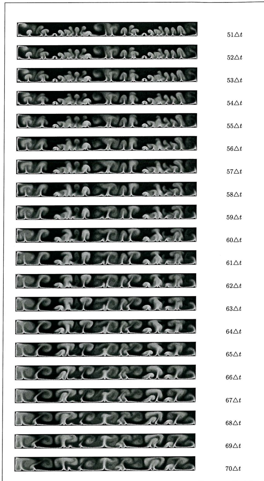
Figure 6.7: Part II: Mixing of Görtler vortices phase, Re = 5 \times 10^3 , \Delta t = 0.0025 s
