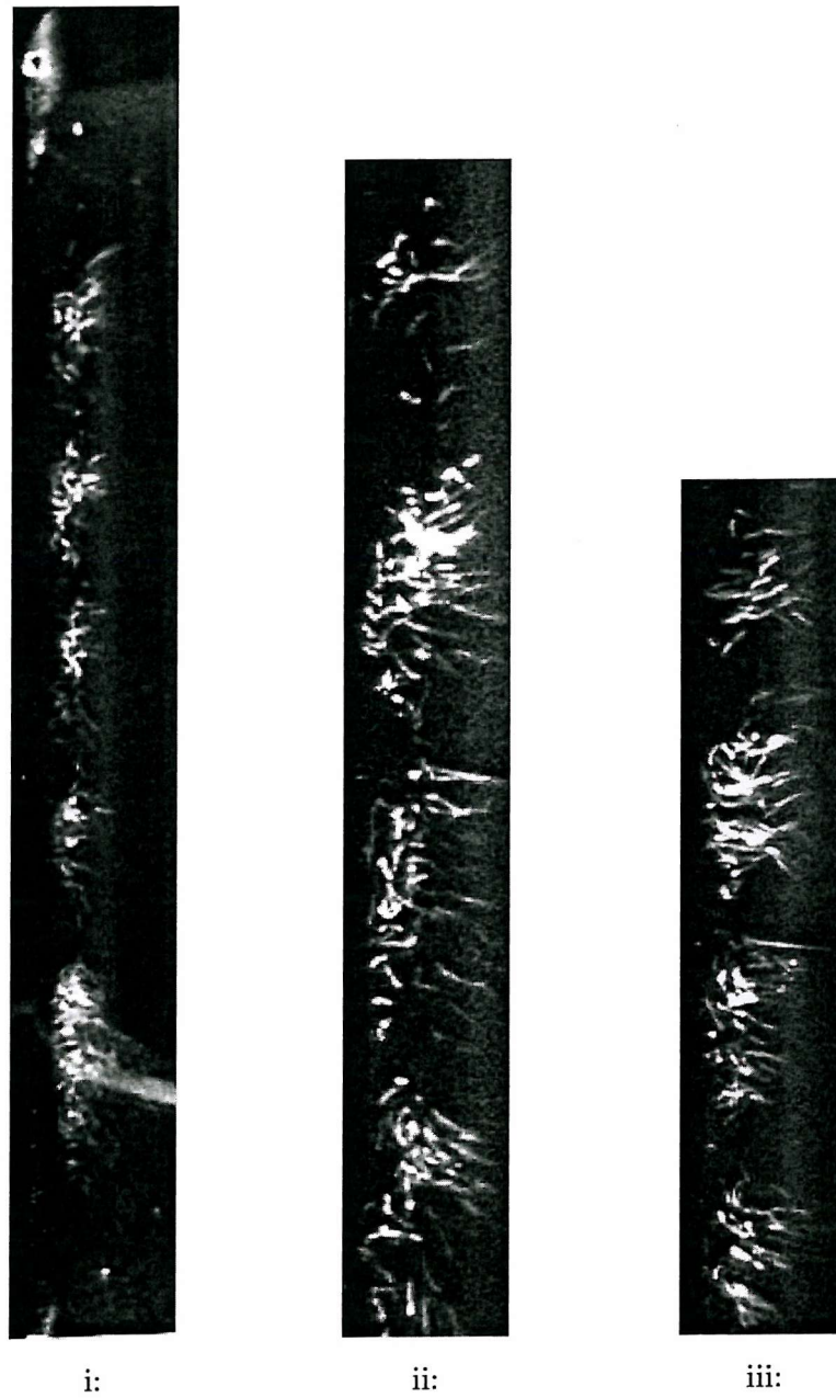
Figure 3.28: Set of three images of bubbles in the experimental rig at a higher bubble flow rate
