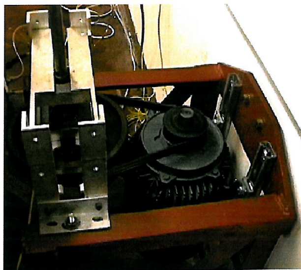
Figure 3.11: Photograph from above of motor framework showing the motor and belt drives
