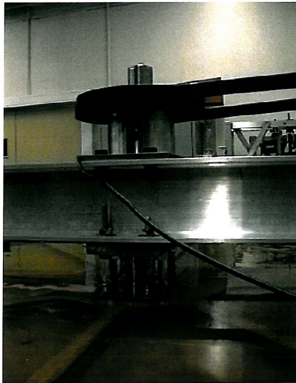
Figure 3.10: Closeup photograph of the top bearing and dynamometer arranged in the rig
