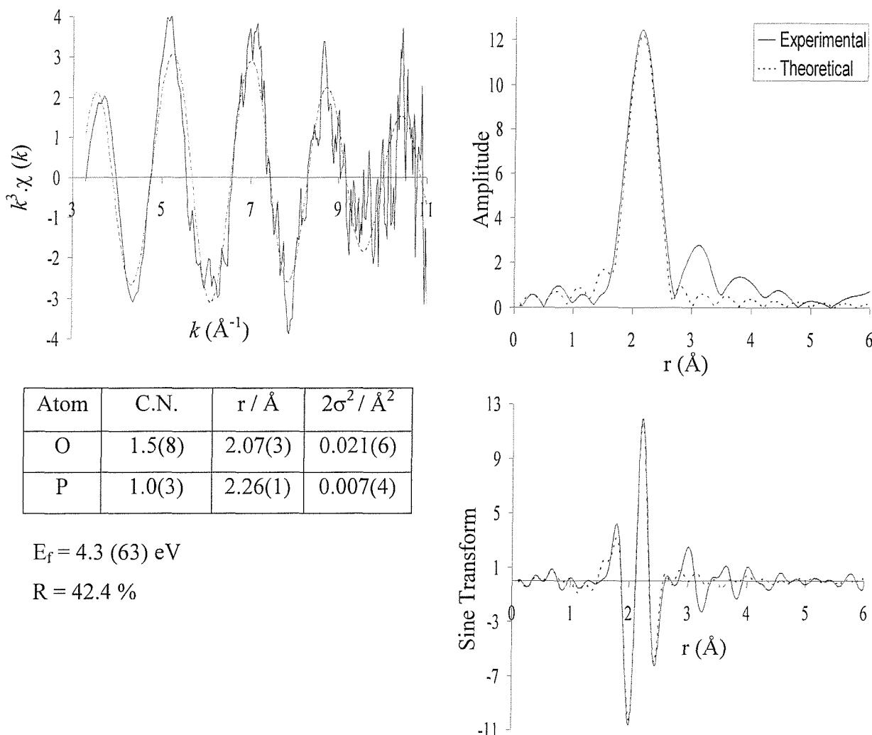
**Figure 3.20** The palladium K-edge  $k^3$ -weighted time resolved EDE data ( $\Gamma^t = 2.2$  ms), Fourier transform and sine transform for the reaction between  $\text{Pd}(\text{OAc})_2$  and  $\text{PCy}_3$  (860 seconds).
