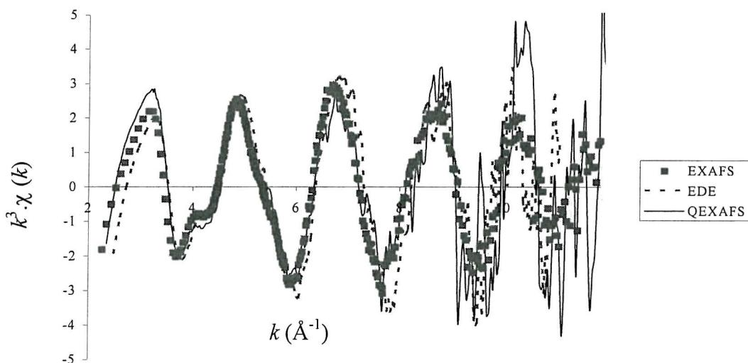
**Figure 3.9** The palladium K-edge  $k^3$ -weighted spectra for species 1 (in solution) comparing spectra quality for EXAFS (1 x 30 minutes), QEXAFS (1 x 12 minutes) and EDE (100 scans, 1.4 ms).
