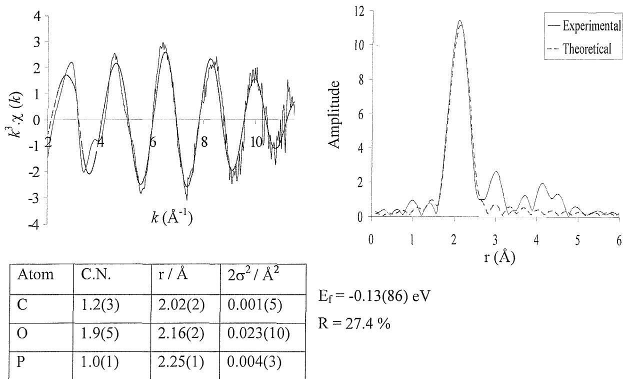
**Figure 3.4 The palladium K-edge  $k^3$ -weighted EXAFS data (2 x 30 minutes) and Fourier transform of species 1 in NMP (RTP).**
