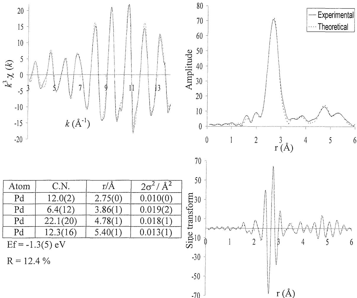
**Figure 2.12 The palladium K-edge  $k^3$ -weighted EXAFS data, Fourier transform and sine transform for an EDE palladium foil at room temperature and pressure (RTP).**
