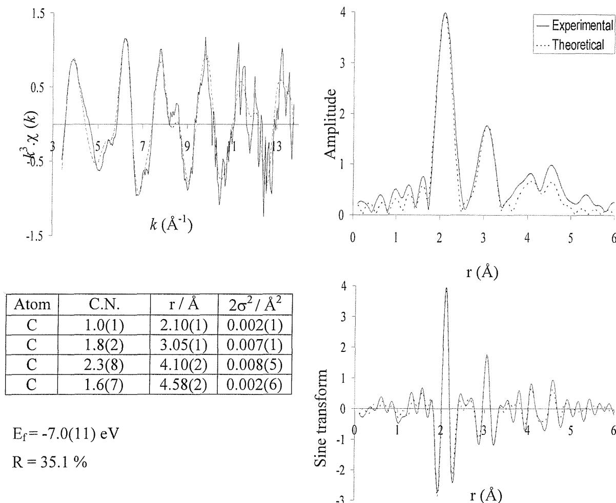
**Figure 4.8** The iodine K-edge  $k^3$ -weighted QEXAFS data (4 x 6 minutes averaged), Fourier transform and sine transform of the PhI Heck reaction, catalysed by **1** (40 °C), after heating to 50 °C.
