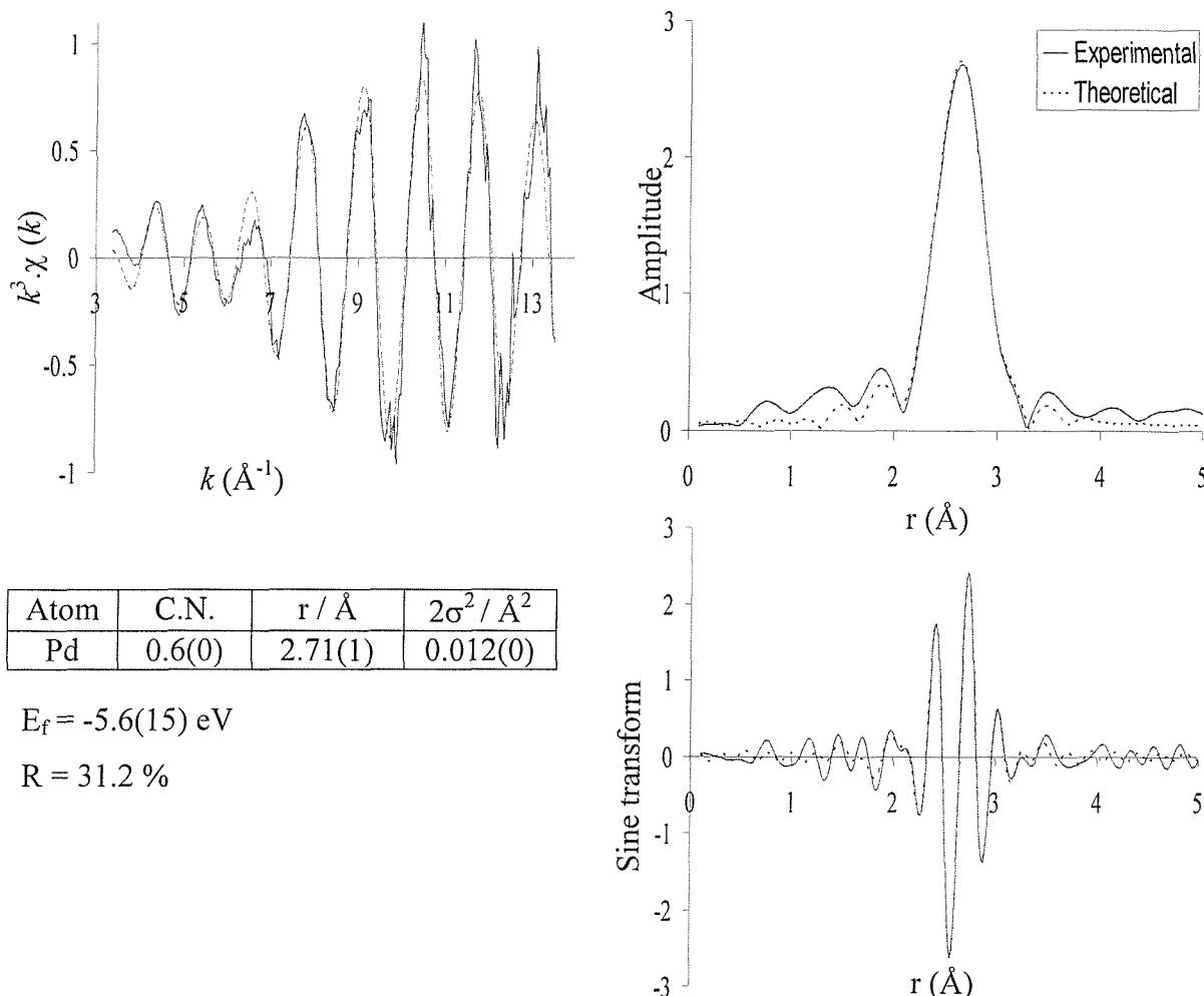
**Figure 4.9** The iodine K-edge  $k^3$ -weighted QEXAFS data (10 x 6 minutes averaged), Fourier transform and sine transform showing the Heck reaction after heating at 115 °C for 2 hours (RTP).
