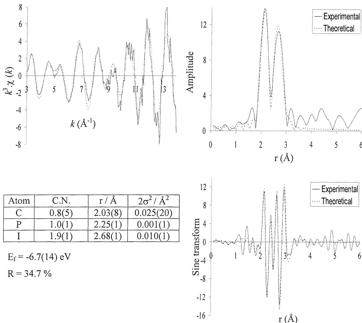
**Figure 4.25** The palladium K-edge  $k^3$ -weighted QEXAFS data (10 x 6 minutes averaged), Fourier transform and sine transform for the reaction between iodobenzene and methallyl alcohol with species 3b as catalyst (RTP) after heating for 2 hours at 130 °C.
