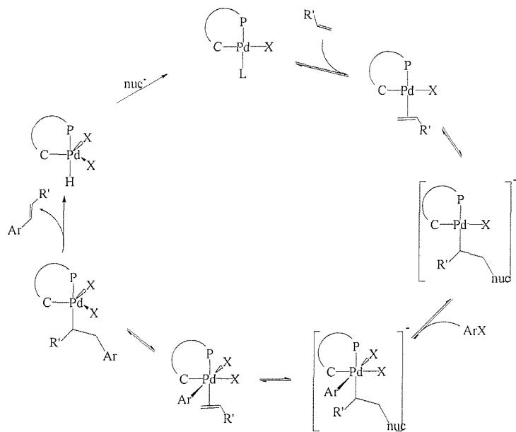
**Figure 1.8** The catalytic cycle proposed by Shaw *et al.*<sup>36</sup> following a palladium (II)-palladium (IV) cycle with a bidentate palladacycle (nuc = nucleophile (Br<sup>-</sup>, OH<sup>-</sup>)).
