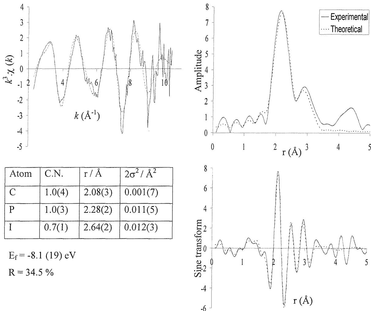
**Figure 5.11** The palladium K-edge  $k^3$ -weighted QEXAFS data (5 x 6 minutes averaged), sine and Fourier transform for the  $\text{Pd}(\text{OAc})_2 / \text{P}^t\text{Bu}_3 / \text{PhI}$  reaction (RTP), solution was homogeneous at room temperature.
