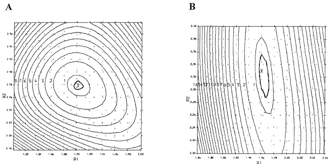
**Figure 2.11 Two-dimensional map of the fit index plotted of two parameters derived from curve fitting, showing a good refinement with a spherical contour (A) and poorly defined variables with contours elongated in one direction (B).**
