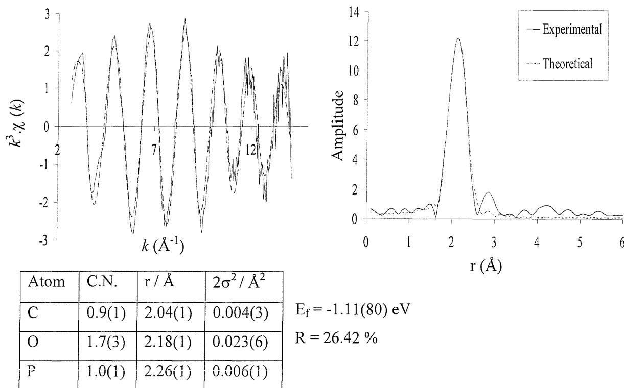
**Figure 3.7 The palladium K-edge  $k^3$ -weighted QEXAFS (6 x 12 minutes, averaged) and Fourier transform for the solid state species 1 in NMP (RTP).**
