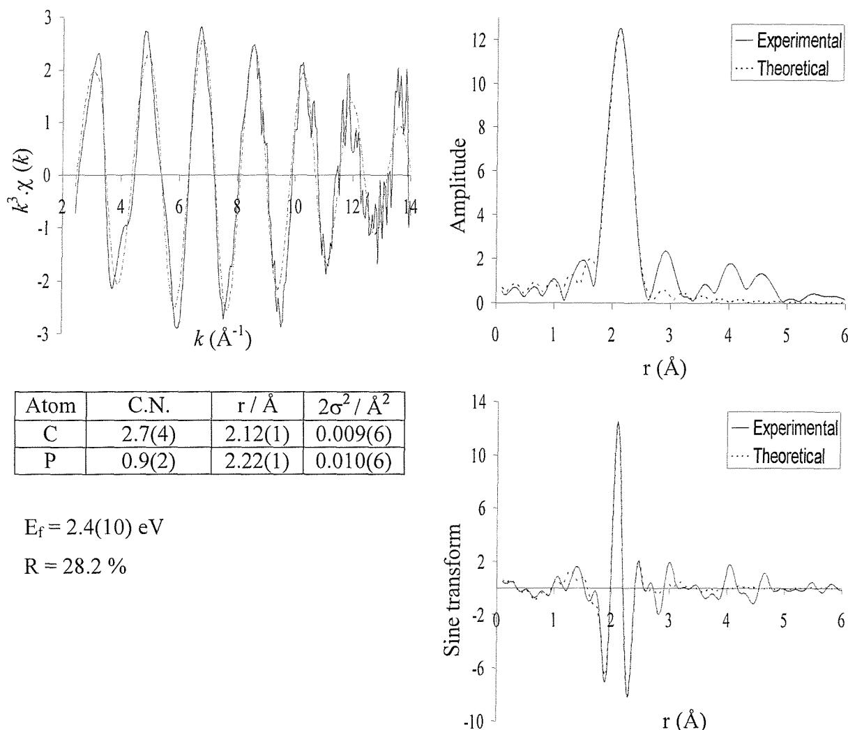
**Figure 4.23** The palladium K-edge  $k^3$ -weighted QEXAFS data (10 x 6 minute averaged), Fourier transform and sine transform of the chlorobenzene reaction (RTP) after heating to 100 °C.
