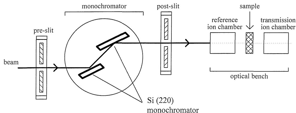
**Figure 2.3 Station 9.2 schematic diagram for transmission mode detection (SRS)<sup>16</sup>**
