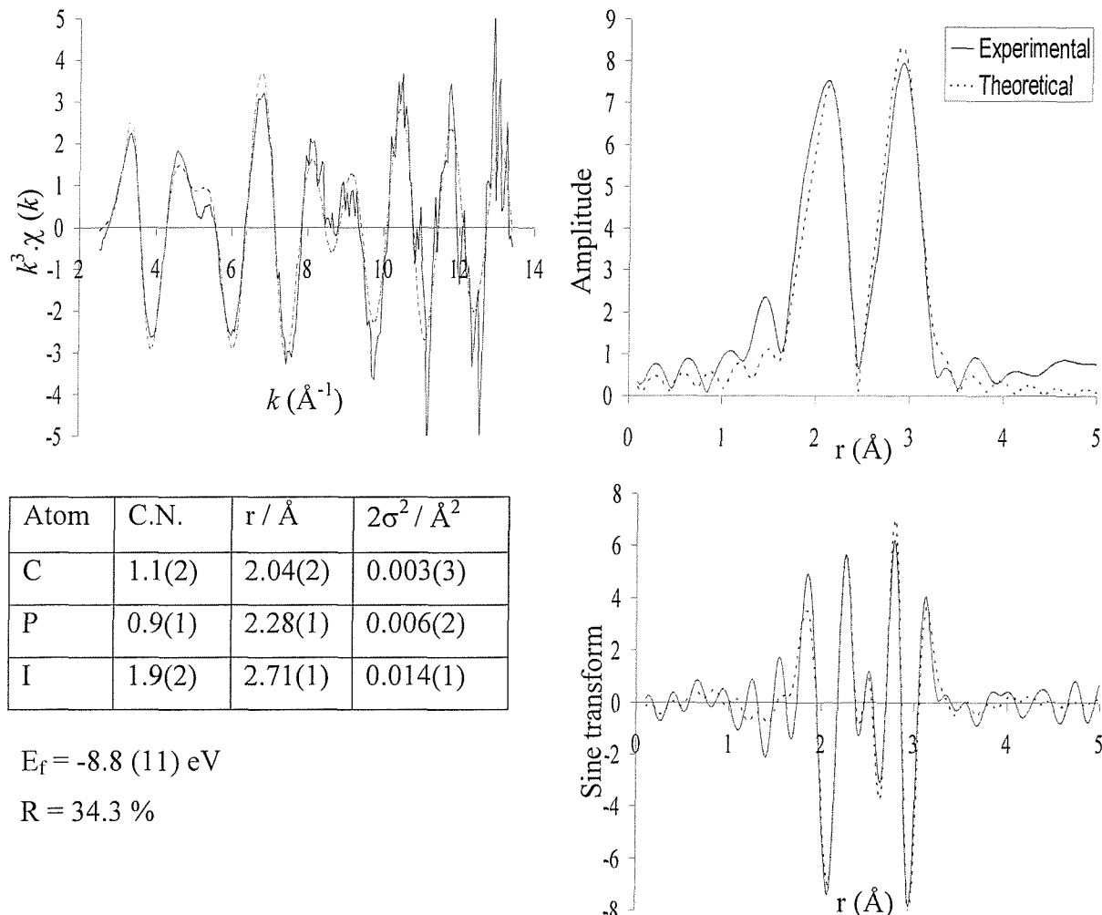
**Figure 5.12** The palladium K-edge  $k^3$ -weighted QEXAFS data (10 x 6 minutes averaged), sine and Fourier transform for the  $\text{Pd(OAc)}_2 / \text{P}^t\text{Bu}_3 / \text{PhI}$  reaction (RTP), after heating for 1.5 hours at 115 °C.
