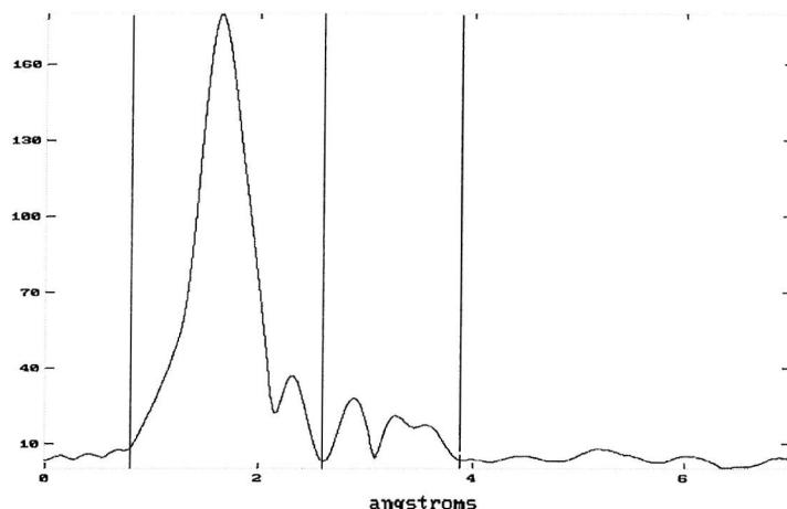
**Figure 3.2 The Fourier transform of the Pd K edge EXAFS (2 x 30 minutes averaged) of species 1 (50 mM) in NMP at room temperature and pressure (RTP), with no phase shift correction.**
