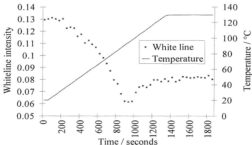
**Figure 3.18** The palladium K-edge white line plot of the reaction between  $\text{Pd}(\text{OAc})_2$  and  $\text{PCy}_3$  (1:3).
