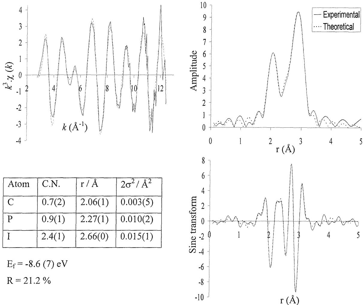
**Figure 5.6** The palladium K-edge  $k^3$ -weighted QEXAFS data (10 x 6 minutes averaged), sine and Fourier transform for the  $\text{Pd(OAc)}_2 / \text{PPh}_3 / \text{PhI}$  reaction (40 °C), after heating for 1.5 hours at 115 °C.
