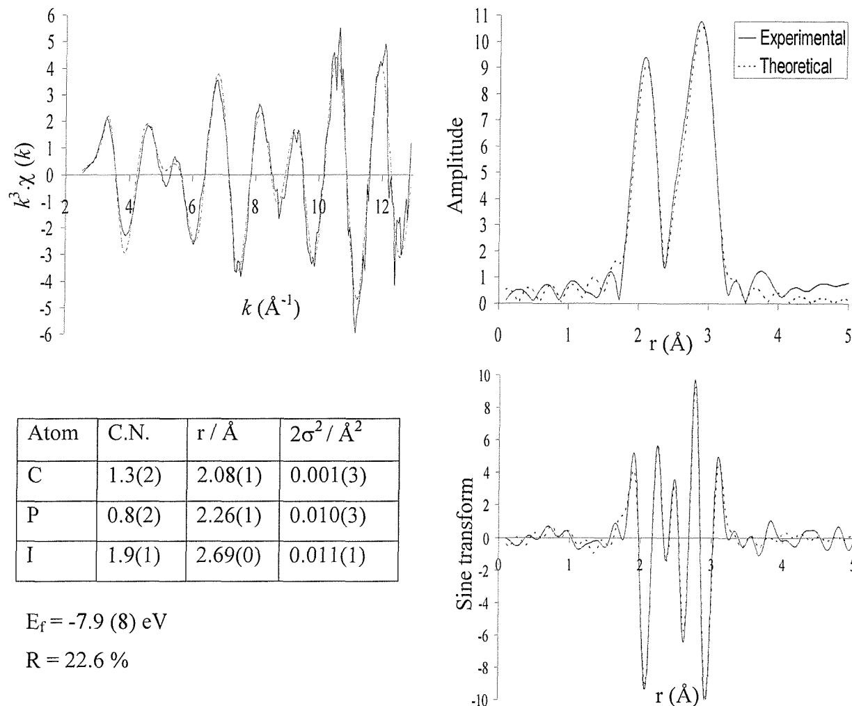
**Figure 5.25** The palladium K-edge  $k^3$ -weighted QEXAFS data (10 x 6 minutes averaged) and Fourier transform for the  $\text{Pd}(\text{OAc})_2 / \text{PNp}_3 / \text{PhI}$  reaction (RTP), after heating at 115 °C for 1.5 hours.
