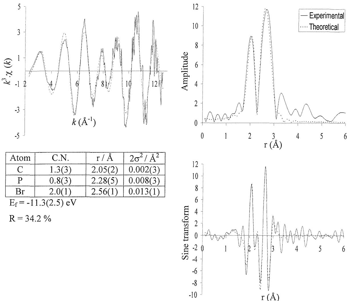
**Figure 4.19** The palladium K-edge  $k^3$ -weighted QEXAFS data (5 x 5 minutes averaged), Fourier transform and sine transform showing the end of the reaction between bromobenzene and methallyl alcohol with species 1 as catalyst (after heating for 2 hours at 115 °C).
