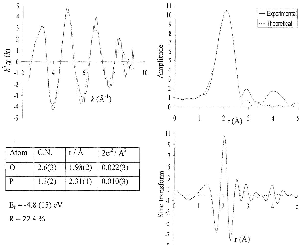
**Figure 5.27** The palladium K-edge  $k^3$ -weighted QEXAFS data (5 x 6 minutes averaged), sine and Fourier transform for the  $\text{Pd}(\text{OAc})_2 / \text{P}(\text{C}_6\text{H}_4(\text{OMe}))_3 / \text{PhI}$  reaction (40 °C), after heating to 40 °C.
