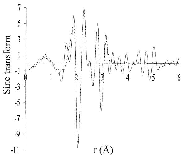
**Figure 4.14 The palladium K-edge  $k^3$ -weighted QEXAFS data and Fourier transform for the Heck reaction, excluding methallyl alcohol (model from table B), after heating for 40 minutes at 115 °C.**
