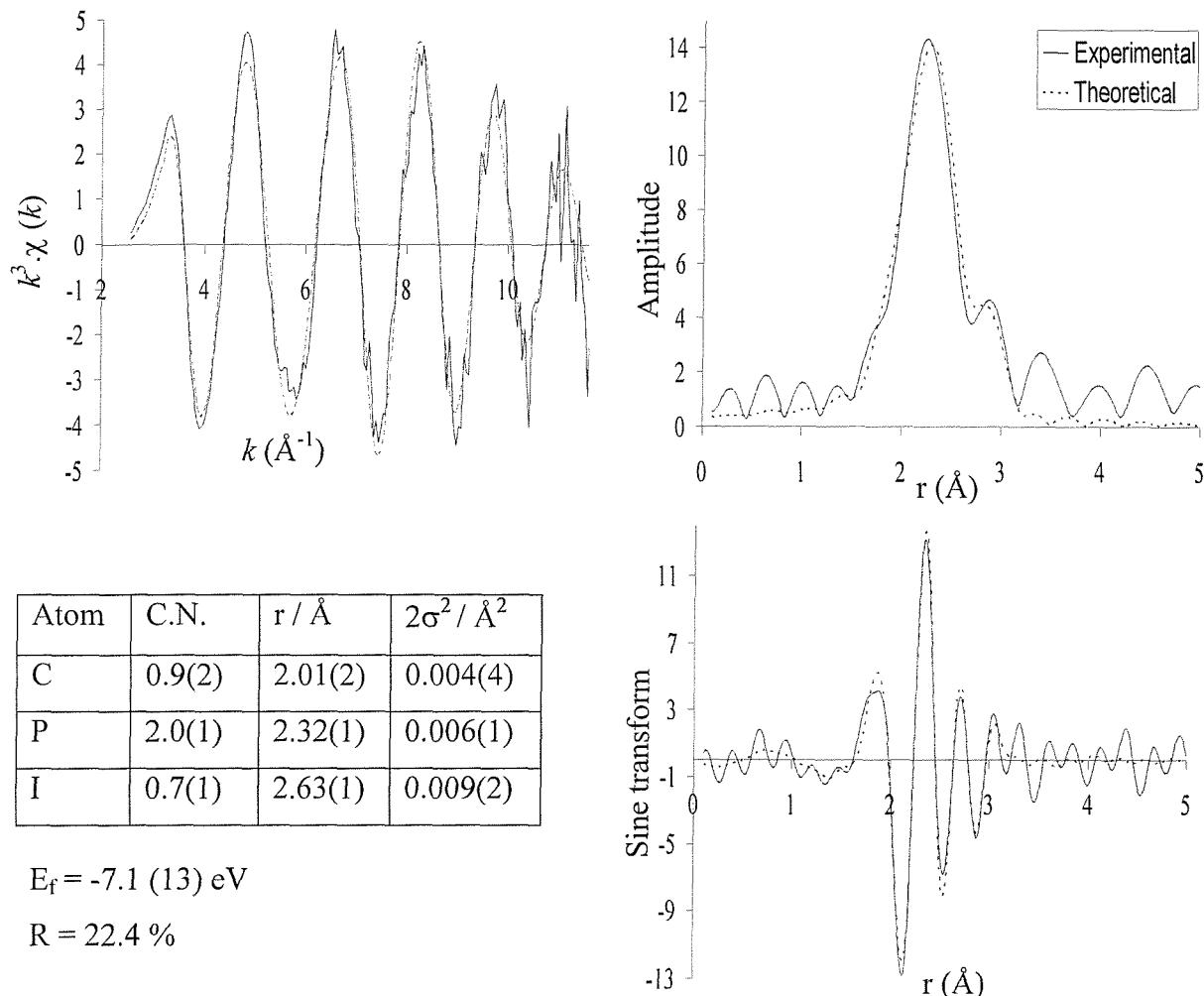
**Figure 5.5 The palladium K-edge  $k^3$ -weighted QEXAFS data (5 x 6 minutes averaged), sine and Fourier transform for the  $\text{Pd}(\text{OAc})_2 / \text{PPh}_3 / \text{PhI}$  reaction (40 °C), after heating to 75 °C.**
