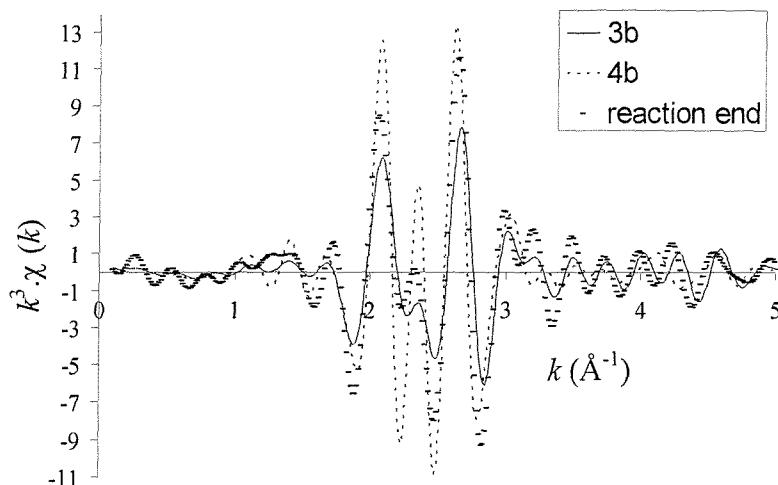
**Figure 4.21 The palladium K-edge sine transform data comparing species **3b** and **4b** with the end of the reaction between bromobenzene and methallyl alcohol.**
