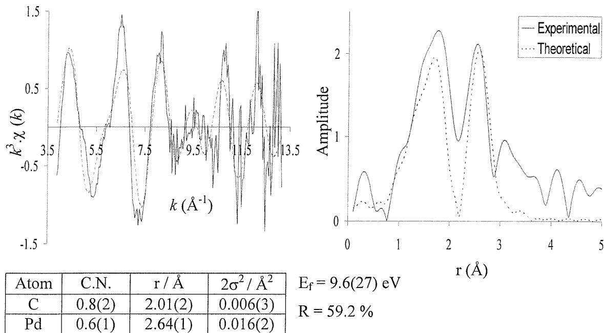
**Figure 4.12** The iodine K-edge  $k^3$ -weighted (1 x 6 minute) QEXAFS data and Fourier transform of the Heck reaction (the scan was started when the reaction was at 65 °C which heated to 115 °C during the duration of the scan).
