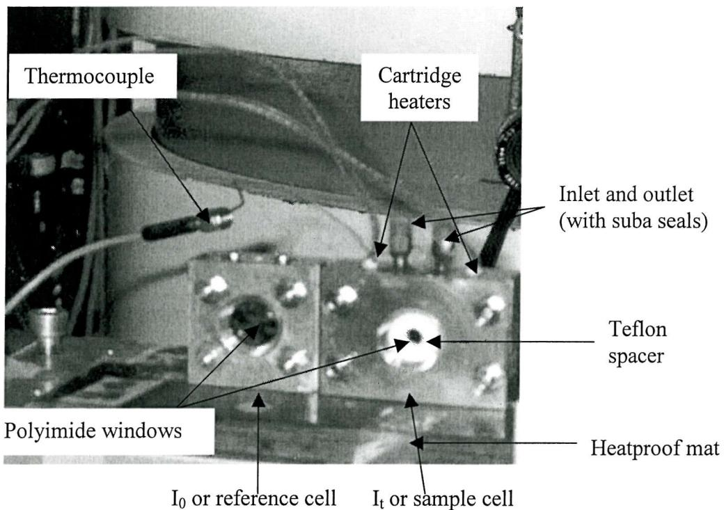
**Figure 2.5 EDE cells arrangement on ID24**
