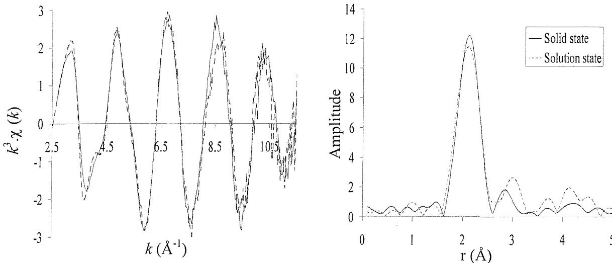
**Figure 3.8 The palladium K-edge  $k^3$ -weighted QEXAFS ( $6 \times 12$  minutes, averaged) of the solid state species **1** compared with the EXAFS ( $2 \times 30$  minutes) for the solution state species **1** in NMP (RTP).**
