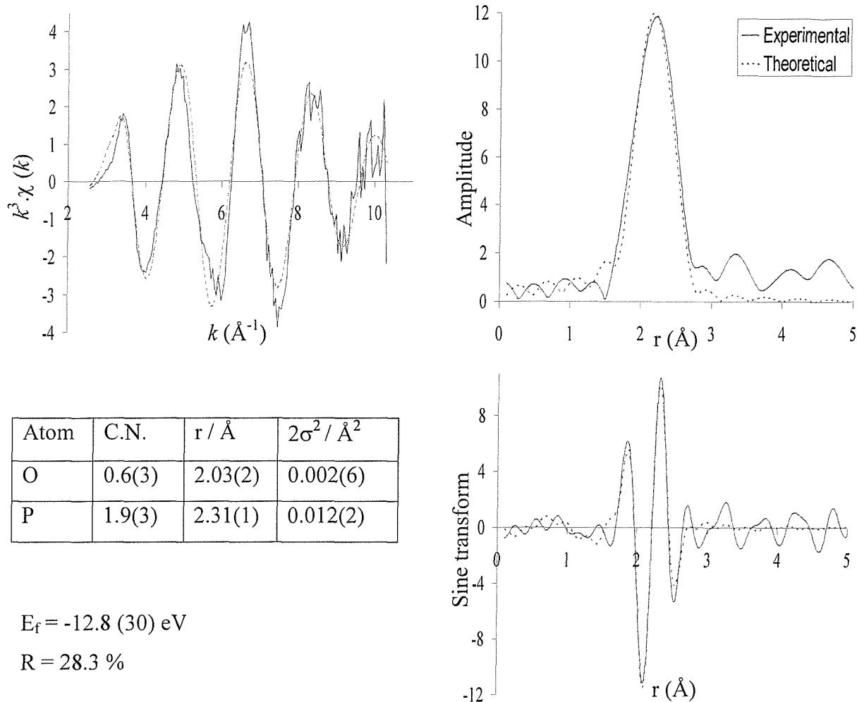
**Figure 5.16** The palladium K-edge  $k^3$ -weighted QEXAFS data (5 x 6 minutes averaged), sine and Fourier transform for the  $\text{Pd}(\text{OAc})_2 / \text{P}^t\text{Bu}_3 / \text{PhCl}$  reaction (RTP), which was homogeneous at room temperature.
