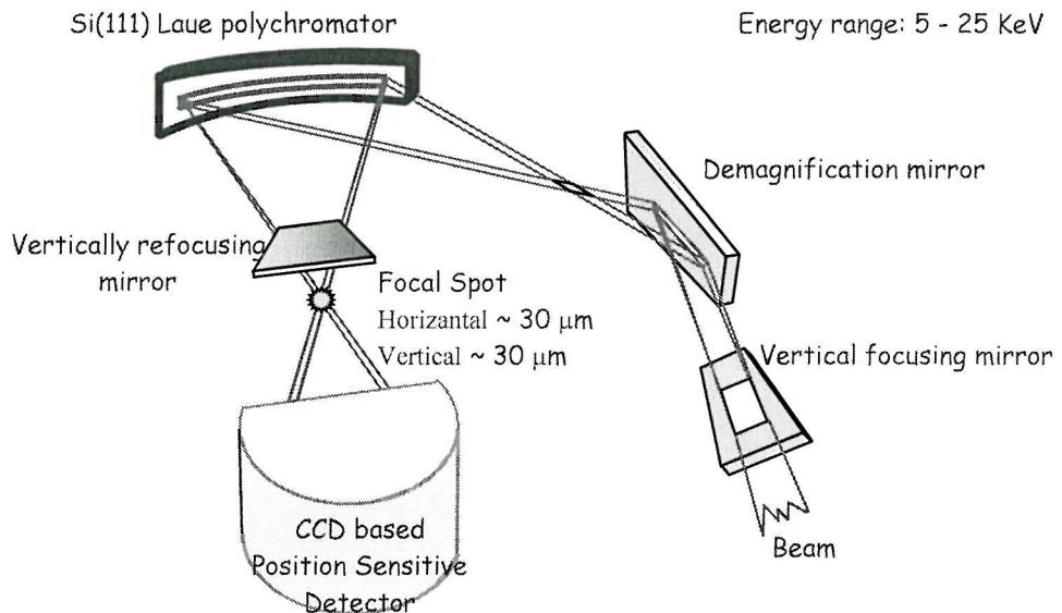
**Figure 2.4 The EDE arrangement on ID24 (Grenoble)<sup>17</sup>**
