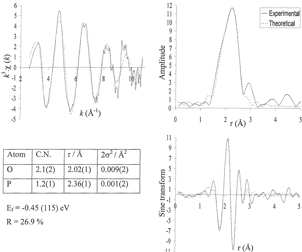
**Figure 5.17** The palladium K-edge  $k^3$ -weighted QEXAFS data (5 x 6 minutes averaged), sine and Fourier transform for the  $\text{Pd}(\text{OAc})_2 / \text{PCy}_3 / \text{PhI}$  reaction (40 °C), after heating to 40 °C.
