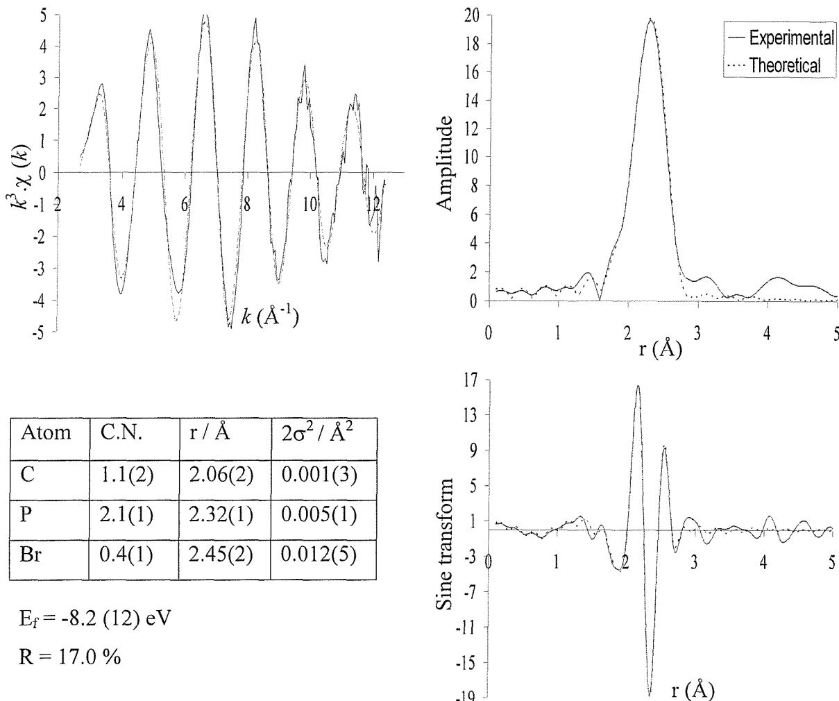
**Figure 5.7** The palladium K-edge  $k^3$ -weighted QEXAFS data (5 x 6 minutes averaged), sine and Fourier transform for the  $\text{Pd}(\text{OAc})_2 / \text{PPh}_3 / \text{PhBr}$  reaction (40 °C), after heating to 75 °C.
