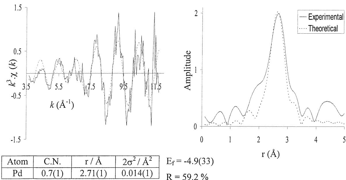
**Figure 4.13** The iodine K-edge  $k^3$ -weighted (1 x 6 minute) QEXAFS data and Fourier transform of the Heck reaction (after heating the sample for 72 minutes at 115 °C).
