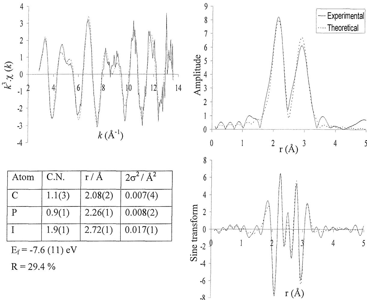
**Figure 5.13** The palladium K-edge  $k^3$ -weighted QEXAFS data (10 x 6 minutes averaged), sine and Fourier transform for the  $\text{Pd}(\text{OAc})_2 / \text{P}^t\text{Bu}_3 / \text{PhI}$  reaction, without alcohol (RTP), after heating for 1.5 hours at 115 °C.
