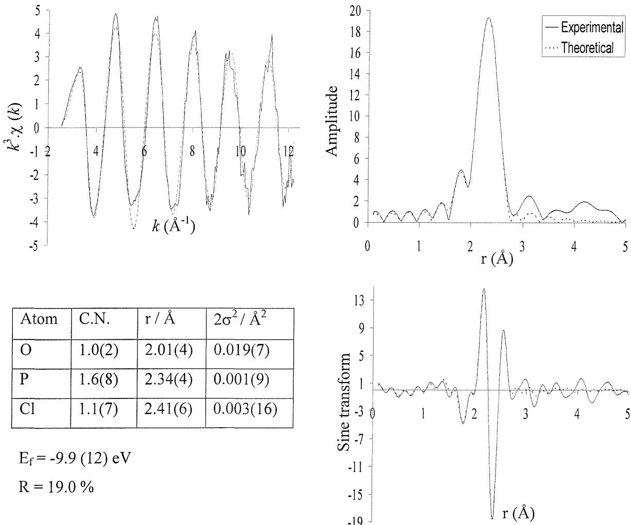
**Figure 5.20** The palladium K-edge  $k^3$ -weighted QEXAFS data (10 x 6 minutes averaged), sine and Fourier transform for the  $\text{Pd}(\text{OAc})_2 / \text{PCy}_3 / \text{PhCl}$  reaction (40 °C), after heating to 115 °C for 20 minutes.
