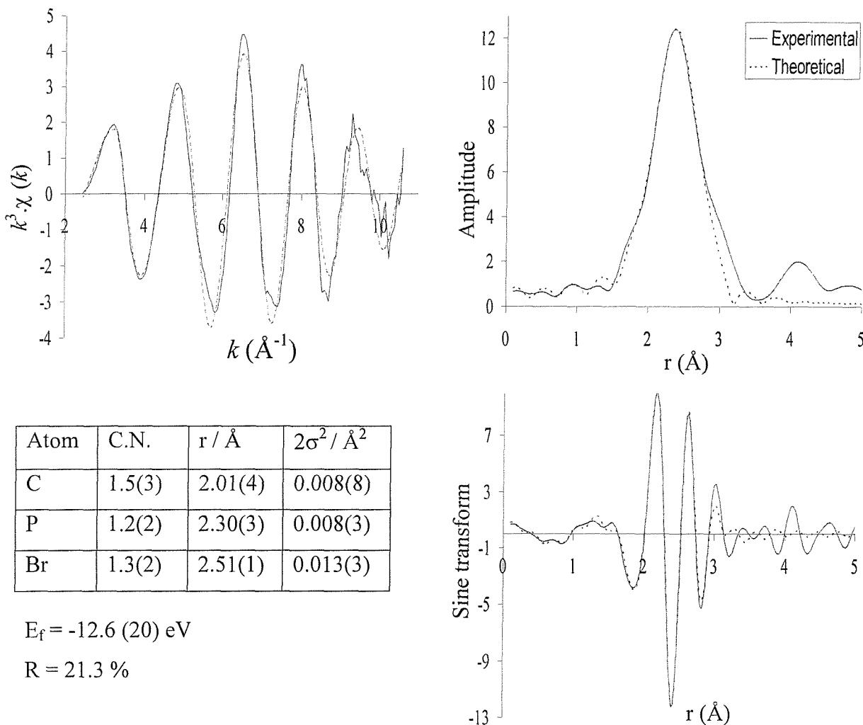
**Figure 5.8** The palladium K-edge  $k^3$ -weighted QEXAFS data (10 x 6 minutes averaged), sine and Fourier transform for the  $\text{Pd(OAc)}_2 / \text{PPh}_3 / \text{PhBr}$  reaction (40 °C), after heating for 1.5 hours at 115 °C.
