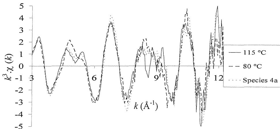
**Figure 4.7b** The palladium K-edge  $k^3$ -weighted EXAFS data, comparing species **4a** with the reaction solution at two stages during the reaction.
