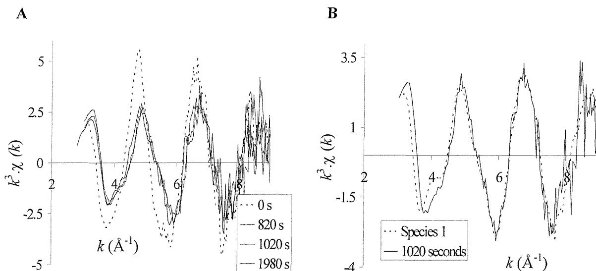
**Figure 3.16** The palladium K-edge  $k^3$ -weighted EDE spectra (50 scans,  $I_t = 1.2$  ms) for the formation of species 1 (A) and the comparison of EDE scan ( $t = 1020$  seconds) with an EXAFS scan of solution state species 1.
