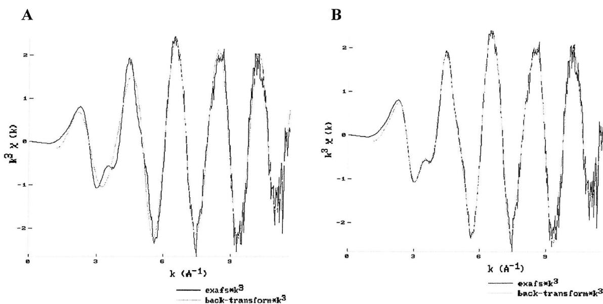
**Figure 3.3 Comparison of  $k^3$  data with  $k^3$  back transformed data for species 1, with back transform limits of 0.80 to 2.60  $\text{\AA}^{-1}$  (A) and 0.80 to 3.88  $\text{\AA}^{-1}$  (B).**
