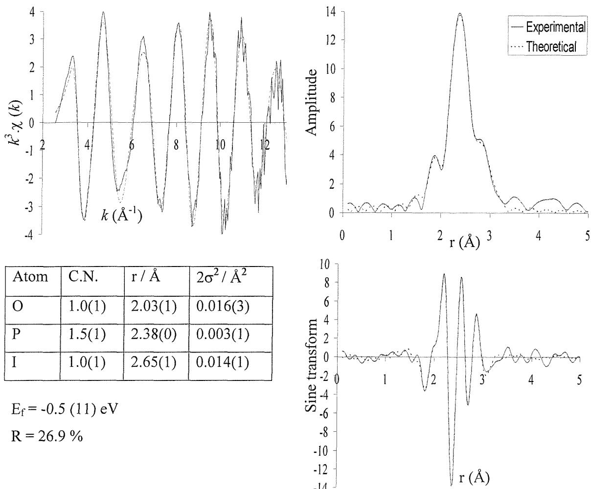
**Figure 5.18** The palladium K-edge  $k^3$ -weighted QEXAFS data (10 x 6 minutes averaged), sine and Fourier transform for the  $\text{Pd}(\text{OAc})_2 / \text{PCy}_3 / \text{PhI}$  reaction (40 °C), 115 °C for 20 minutes.
