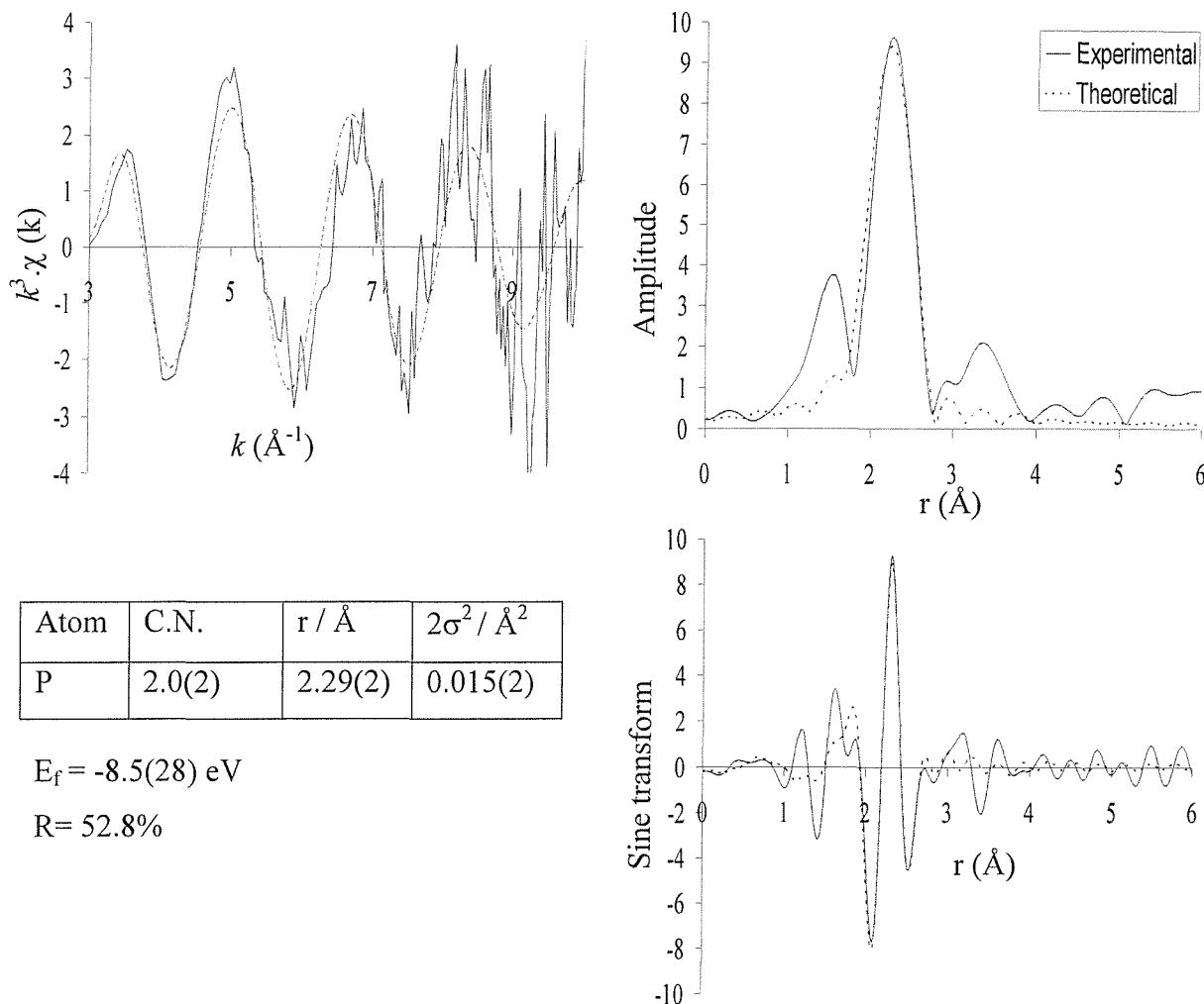
**Figure 3.23 The palladium K-edge  $k^3$ -weighted EDE time resolved data ( $I^t = 2.2 \text{ ms}$ ), Fourier transform and sine transform for the reaction between  $\text{Pd}(\text{OAc})_2$  and  $\text{P}^t\text{Bu}_3$  (1:3) (1804 seconds).**
