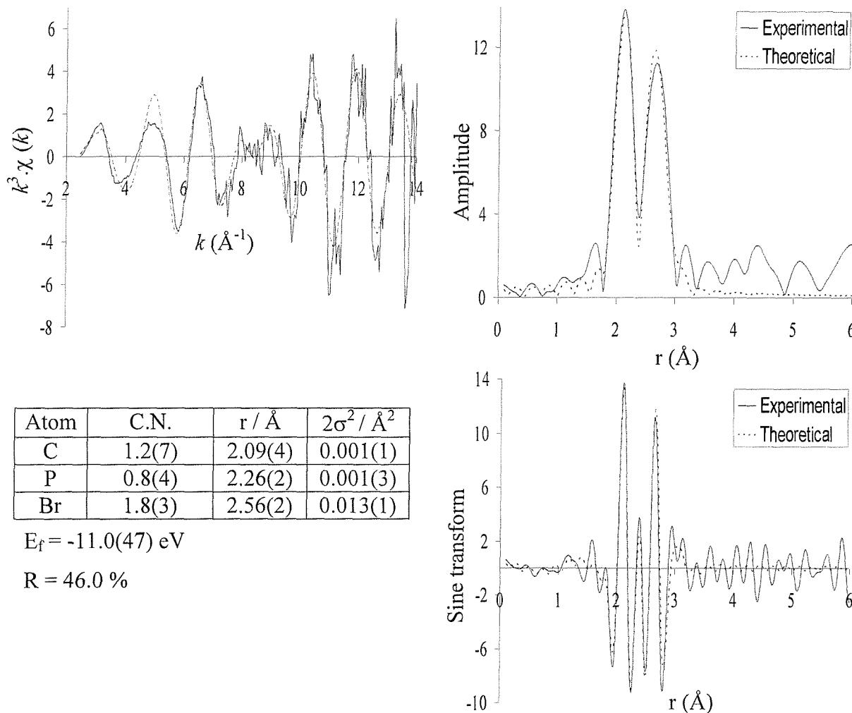
**Figure 4.24** The palladium K-edge  $k^3$ -weighted QEXAFS data (5 x 6 minutes averaged), Fourier and sine transform for the reaction between iodobenzene and methallyl alcohol with species 3b as catalyst (RTP), after heating to 125 °C.
