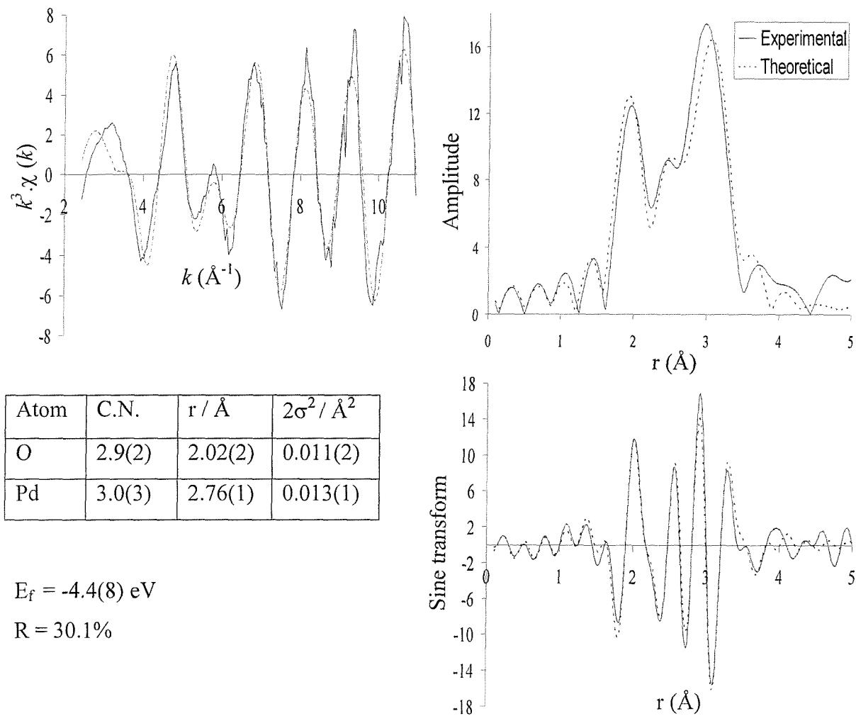
**Figure 5.3 The palladium K-edge  $k^3$ -weighted QEXAFS data (5 x 6 minutes averaged), sine and Fourier transform for the PhBr reaction (RTP), after heating to 40 °C.**
