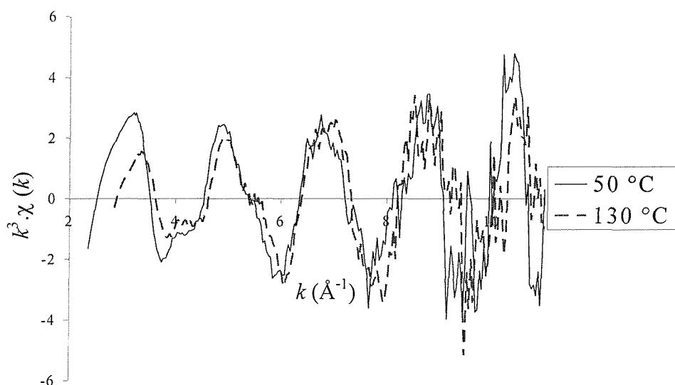
**Figure 3.10** The palladium K-edge  $k^3$ -weighted EXAFS (1 x 30 minutes) of the solution state species 1 NMP (heating).
