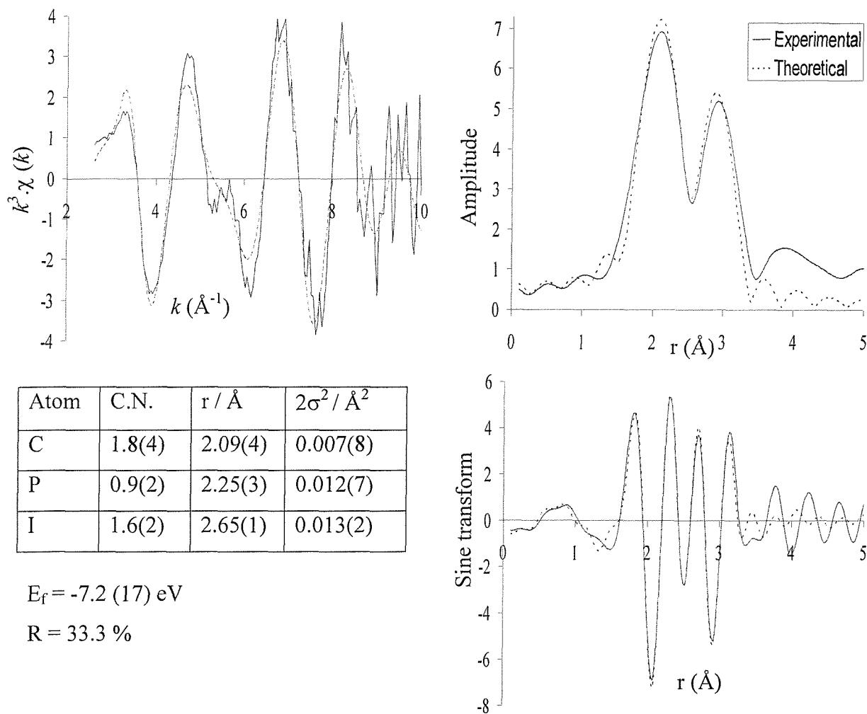
**Figure 5.28** The palladium K-edge  $k^3$ -weighted QEXAFS data (10 x 6 minutes averaged), sine and Fourier transform for the  $\text{Pd}(\text{OAc})_2 / \text{P}(\text{C}_6\text{H}_4(\text{OMe}))_3 / \text{PhI}$  reaction (RTP), after heating for 1.5 hours at 115 °C.
