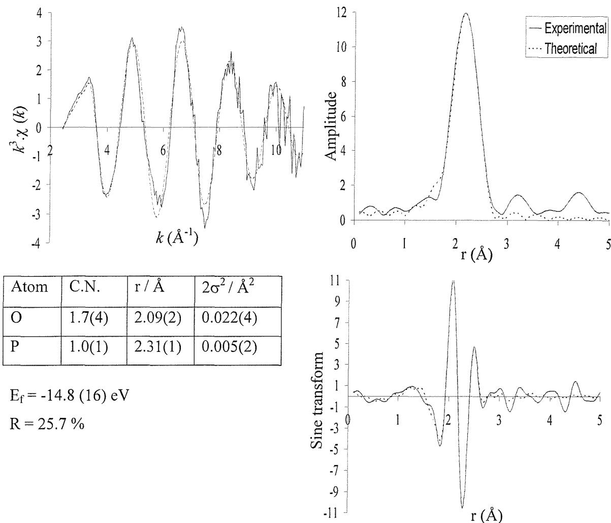
**Figure 5.14** The palladium K-edge  $k^3$ -weighted QEXAFS data (5 x 6 minutes averaged), sine and Fourier transform for the start of the  $\text{Pd}(\text{OAc})_2 / \text{P}^t\text{Bu}_3 / \text{PhBr}$  reaction (RTP), which was homogeneous at room temperature.
