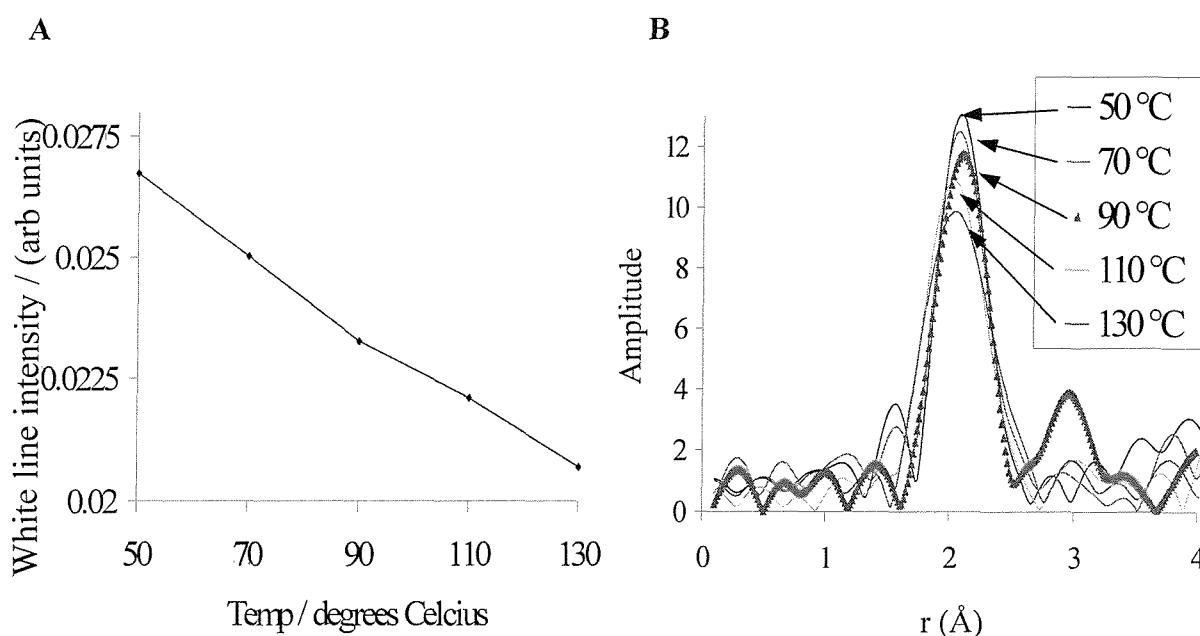
**Figure 3.11** Graph of the normalised white line intensity for species 1 against temperature (A) and the palladium K-edge  $k^3$ -weighted QEXAFS and Fourier transforms (1 x 12 minutes) (B) for species 1 on heating to 130 °C.
