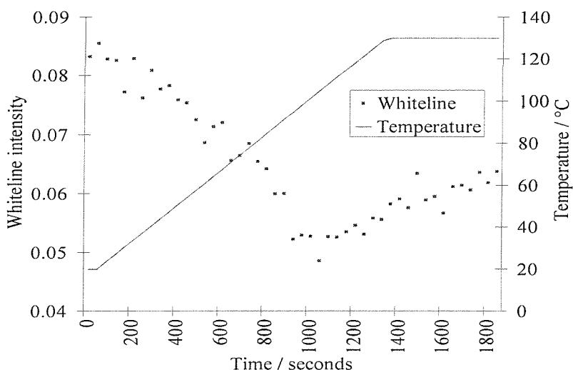
**Figure 3.21** The palladium K-edge white line plot taken during the reaction between  $\text{Pd}(\text{OAc})_2$  and  $\text{P}^t\text{Bu}_3$  (1:3).
