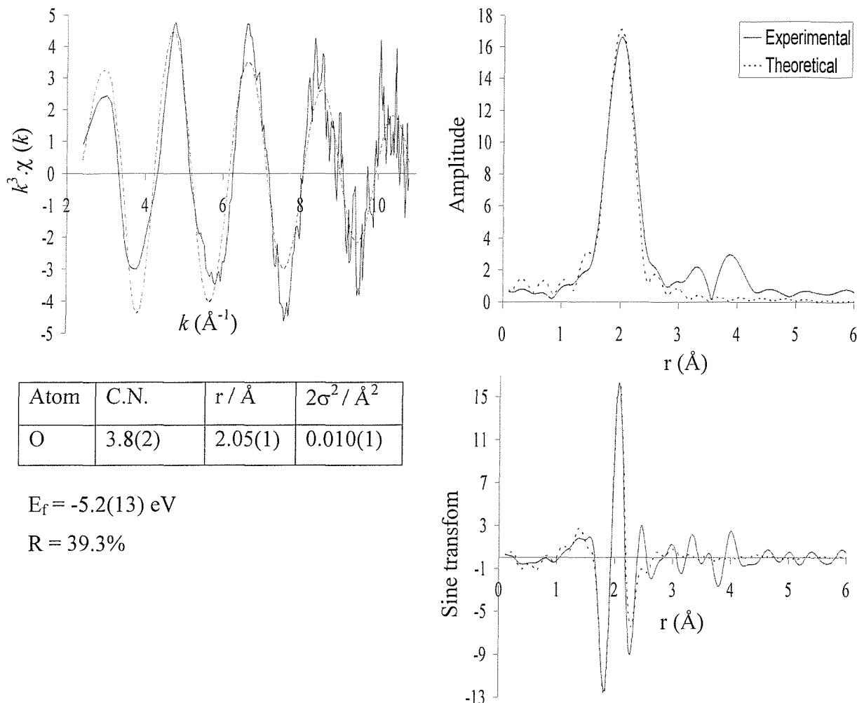
**Figure 3.19** The palladium K-edge  $k^3$ -weighted EDE data ( $I^t = 2.2 \text{ ms}$ ), Fourier transform and sine transform for the reaction between  $\text{Pd}(\text{OAc})_2$  and  $\text{PCy}_3$  (1:3) (0 seconds).
