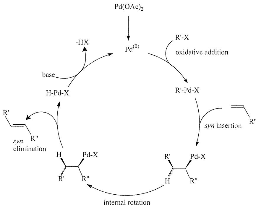
**Figure 1.5 The Heck reaction catalysed by palladium acetate**
