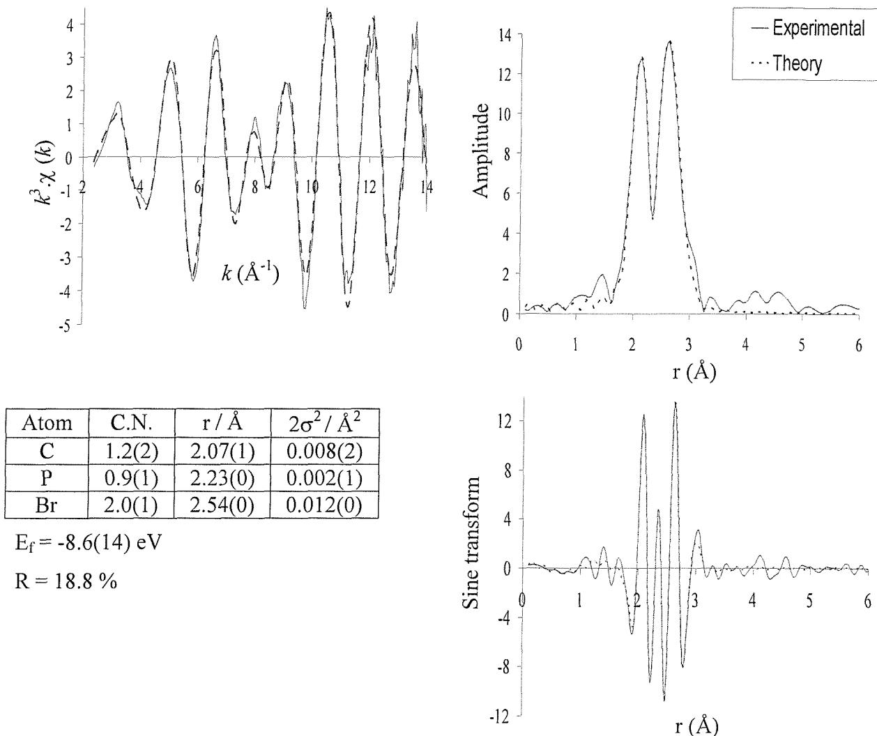
**Figure 4.3** The palladium K-edge  $k^3$ -weighted QEXAFS data (10 x 6 minutes averaged), Fourier transform and sine transform for species 4b (RTP).
