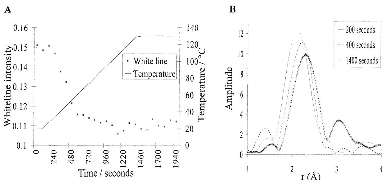
Figure 3.25 The palladium K-edge EDE ( $I^t = 2.2$  ms) white line plot (A) and the corresponding Fourier transform after 200, 400 and 1400 seconds (B).
