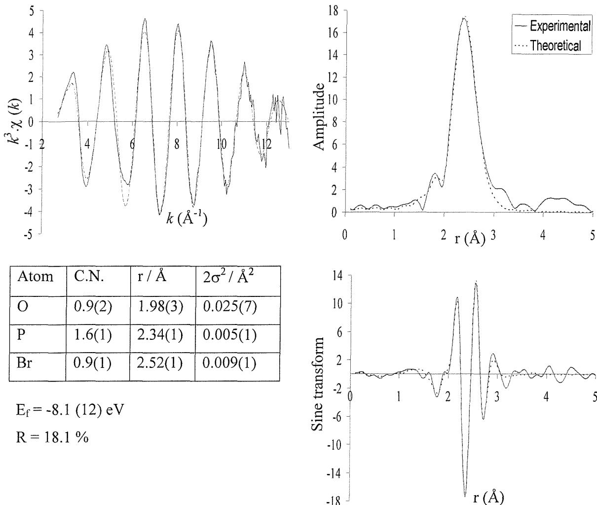
**Figure 5.19** The palladium K-edge  $k^3$ -weighted QEXAFS data (10 x 6 minutes averaged), sine and Fourier transform for the  $\text{Pd}(\text{OAc})_2 / \text{PCy}_3 / \text{PhBr}$  reaction (40 °C), after heating to 115 °C for 20 minutes.
