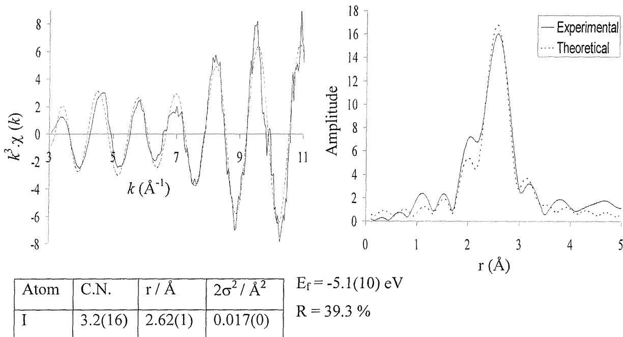
**Figure 5.1** The palladium K-edge  $k^3$ -weighted EDE (100 scans,  $I^t = 6.5 \text{ ms}$ ) for the precatalytic species (RTP).
