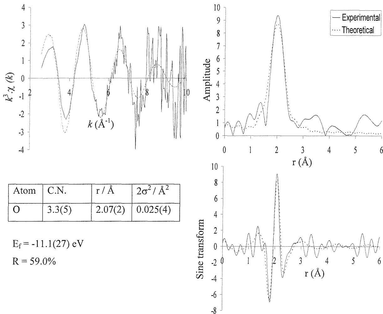
**Figure 3.22 The palladium K-edge  $k^3$ -weighted EDE time resolved data ( $T^t = 2.2 \text{ ms}$ ), Fourier transform and sine transform for the reaction between  $\text{Pd}(\text{OAc})_2$  and  $\text{P}'\text{Bu}_3$  (1:3) (0 seconds).**
