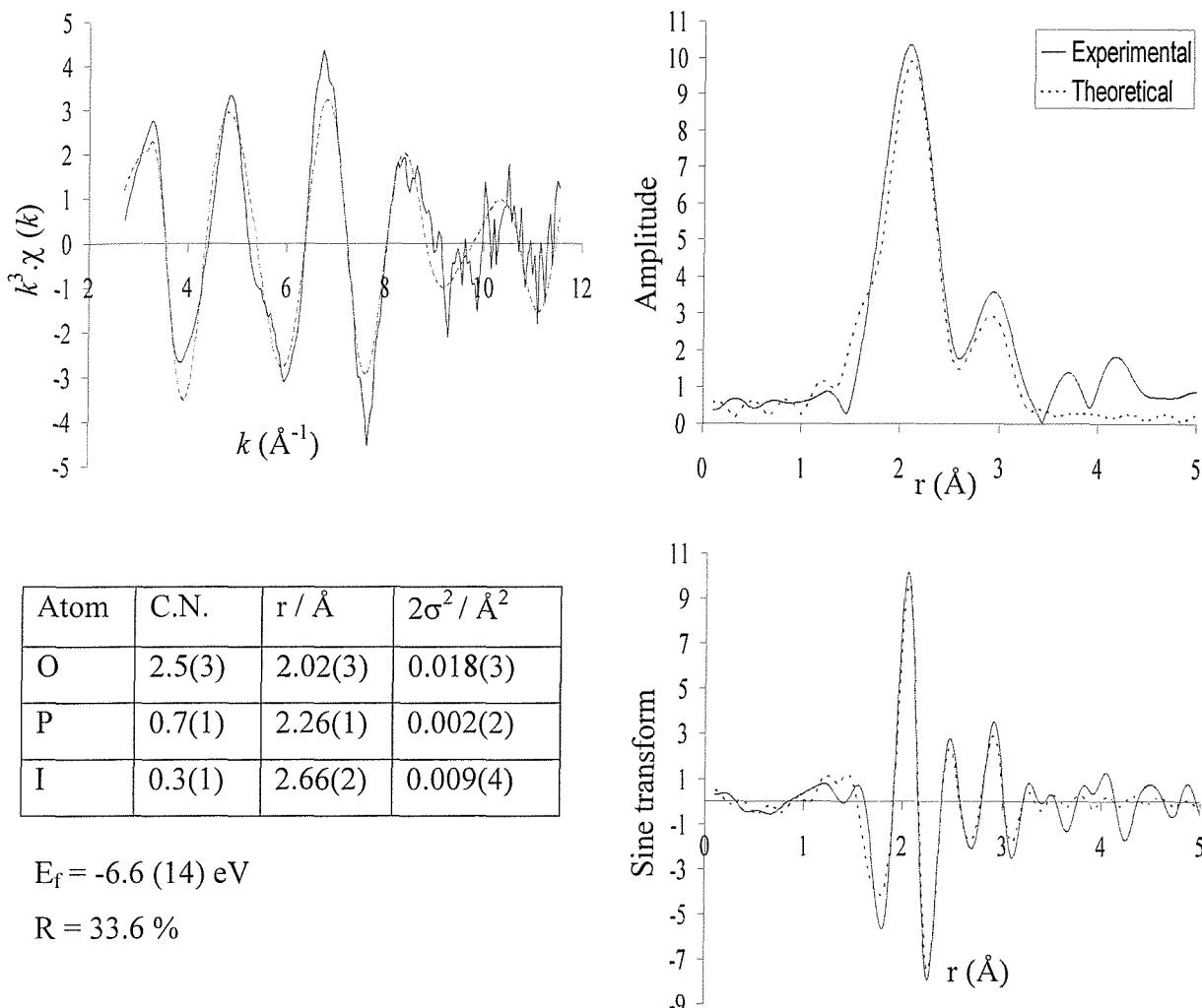
**Figure 5.24** The palladium K-edge  $k^3$ -weighted QEXAFS data (10 x 6 minutes averaged), sine and Fourier transform for the  $\text{Pd}(\text{OAc})_2 / \text{PNp}_3 / \text{PhI}$  reaction ( $40^\circ\text{C}$ ), after heating to  $40^\circ\text{C}$ .
