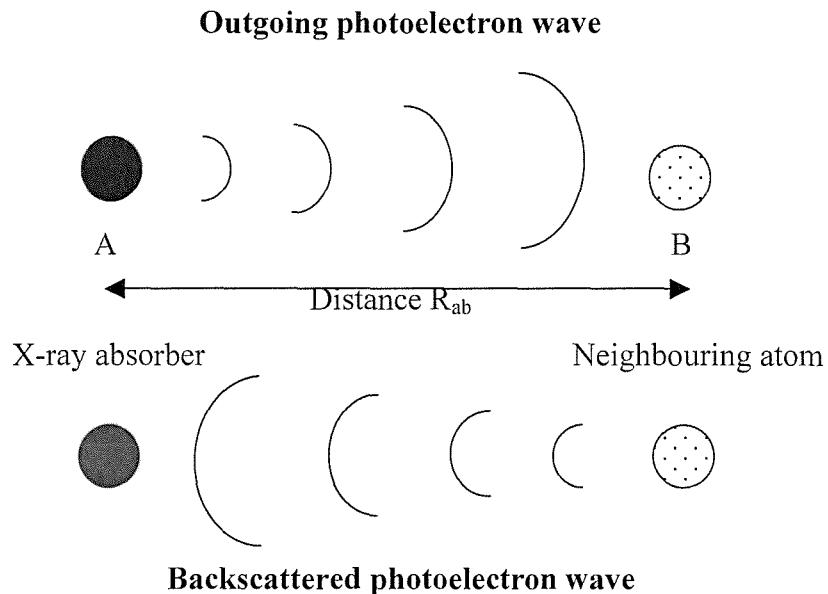
**Figure 2.2 The photoelectron wave emitted from the X-ray absorber and its backscattered portion.<sup>12</sup>**
