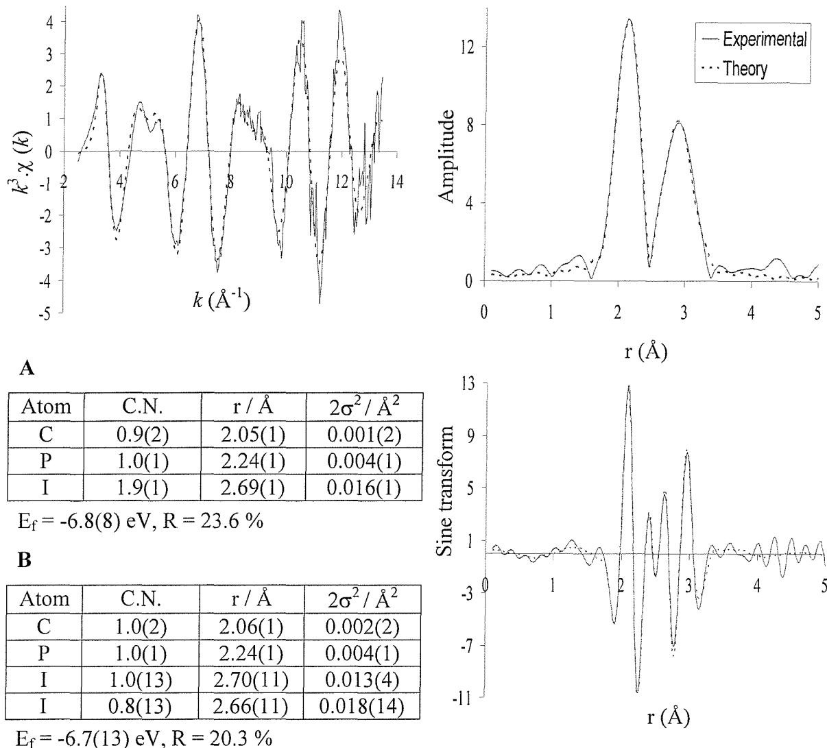
**Figure 4.5** The palladium K-edge  $k^3$ -weighted QEXAFS data (5 x 5 minutes averaged), Fourier transform and sine transform for species 4a in NMP at RTP (modelled on table A).
