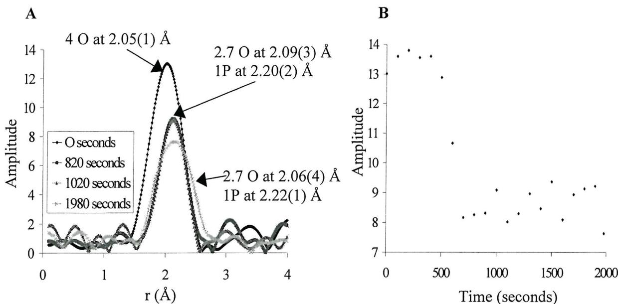
**Figure 3.15** The palladium K-edge Fourier transforms for selected times during the formation of species **1** (A) and the Fourier transform peak heights (showing every five spectra) for the same reaction (B).
