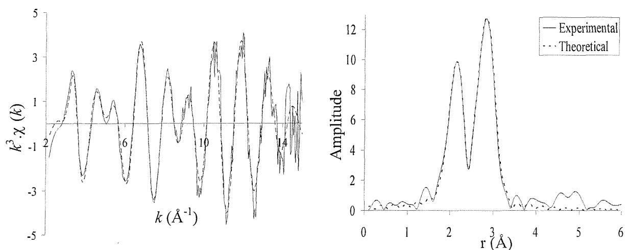
**Figure 4.7** The palladium K-edge  $k^3$ -weighted QEXAFS data and Fourier transform of the reaction between iodobenzene and methallyl alcohol, with species 1 as catalyst (50 mM).
