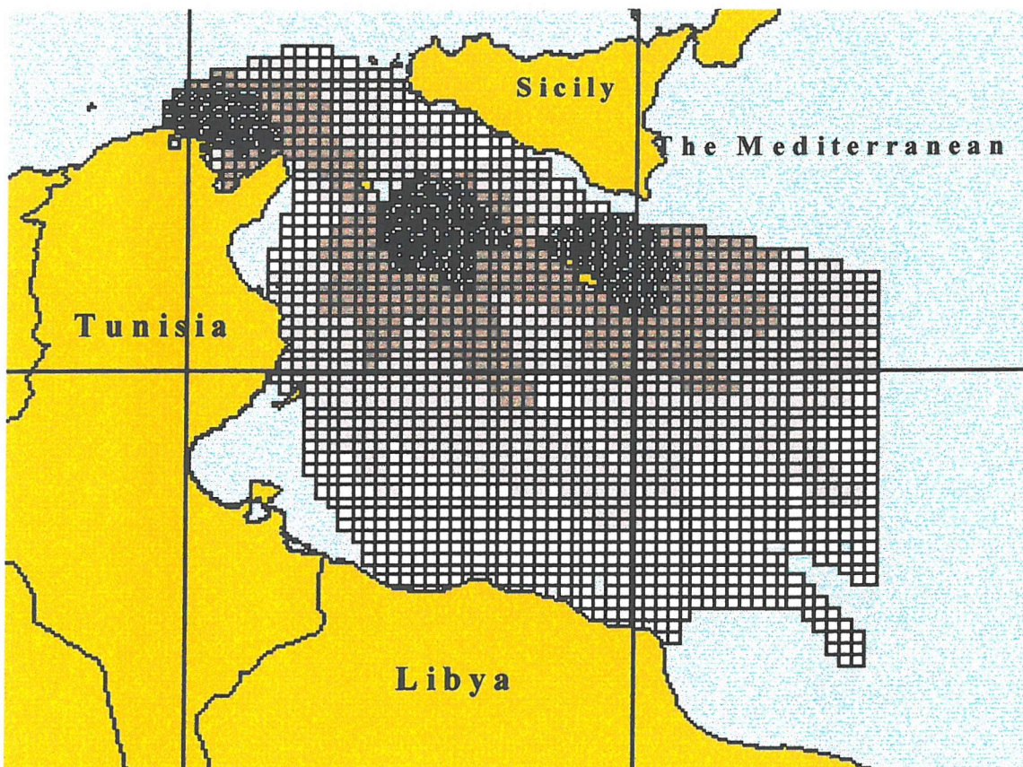
Figure 6.1 The area of influence of three simulated release sites in the Sicily- Malta channel (Not to scale)(World Bank, 1998).
