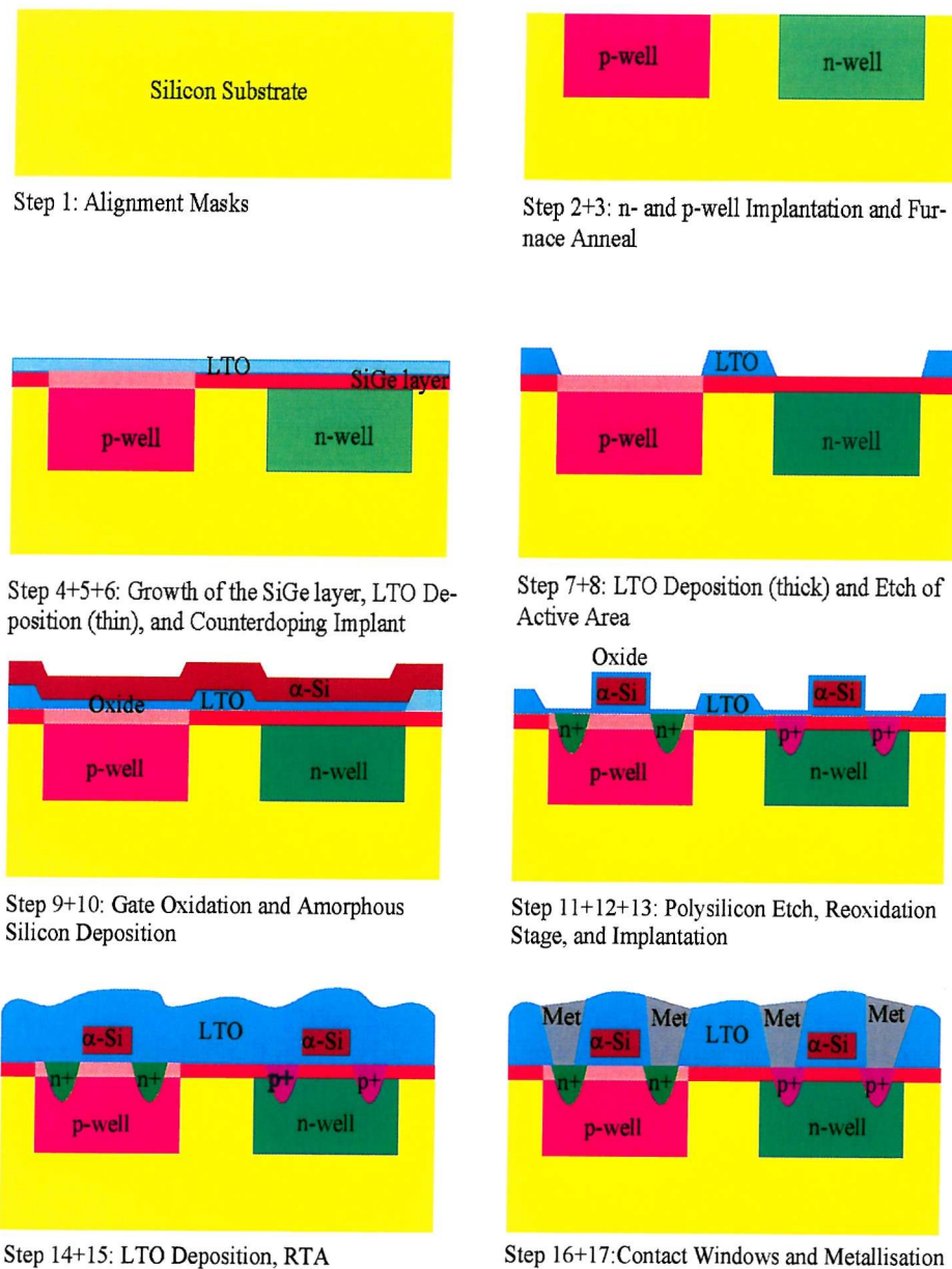
Figure 7.1: Schematic representation of the pseudomorphic SiGe CMOS process, the dimensions are not to scale
