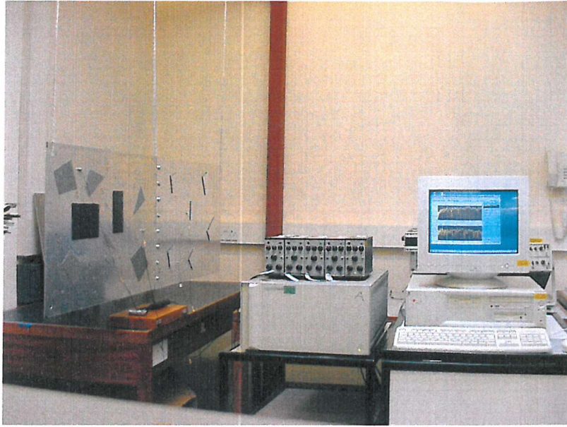
Figure 7.9. Experimental configuration for the measurement of vibrational energy and input force.
