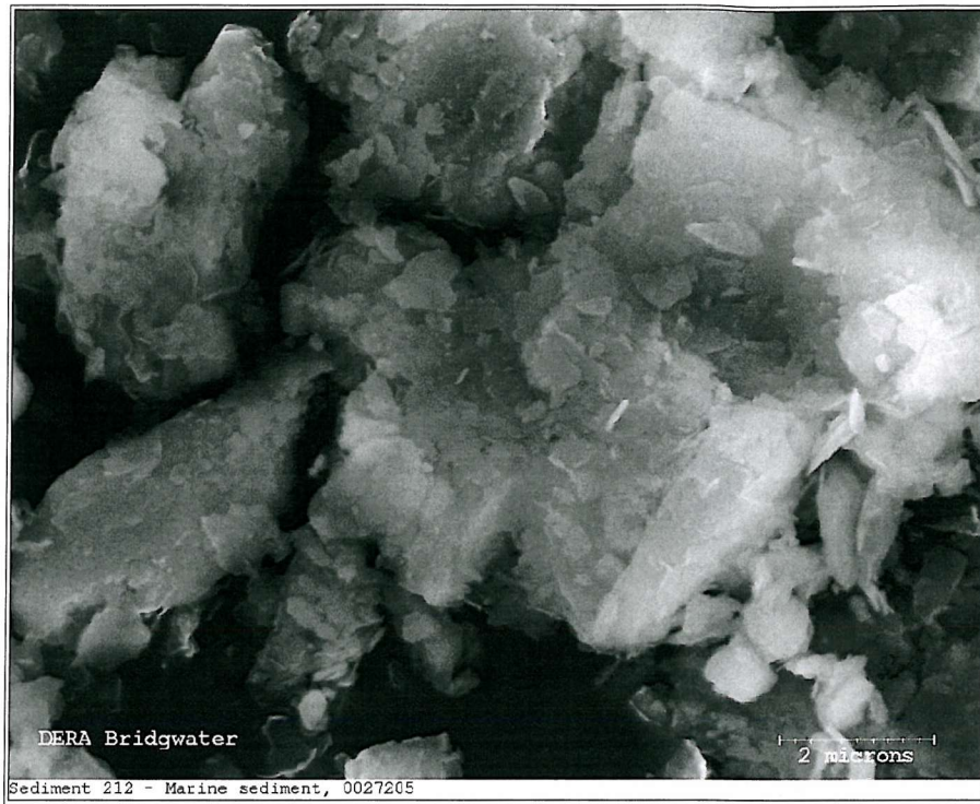
Figure 6.29. Scanning electron micrograph of sediment particles taken with an original instrument magnification of \times 10000 - detail of the area shown in Figure 6.28.
