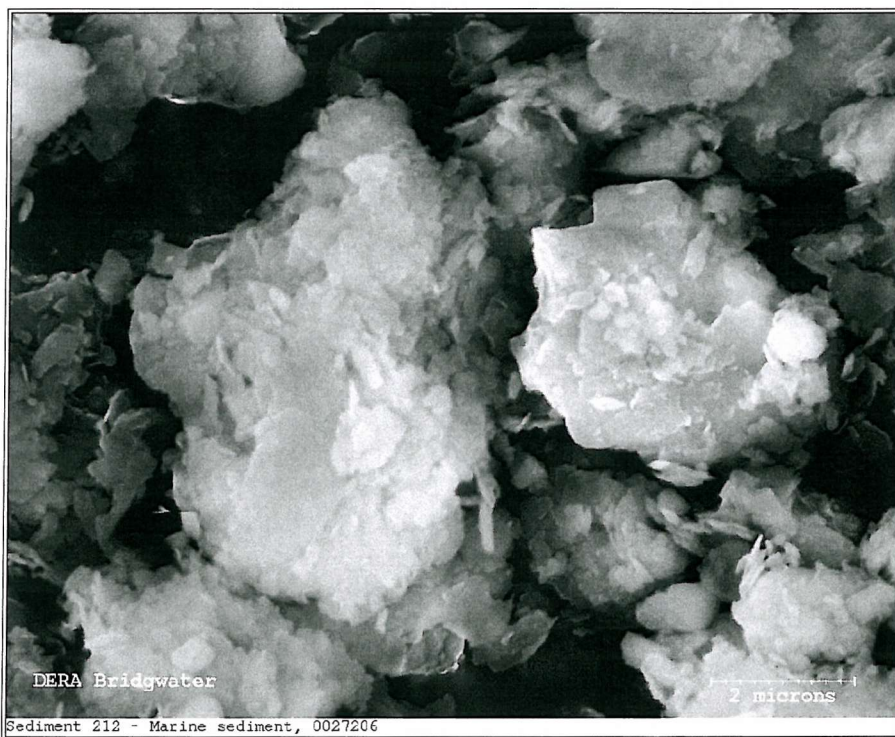
Figure 6.30. Scanning electron micrograph of sediment particles taken with an original instrument magnification of \times 10000 - another detail of the area shown in Figure 6.28.
