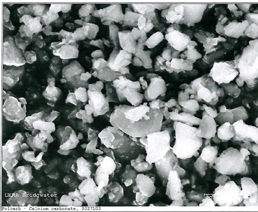
Figure 6.23. Scanning electron micrograph of Polcarb particles taken with an original instrument magnification of \times 10000 - another detail of area shown in Figure 6.21.
