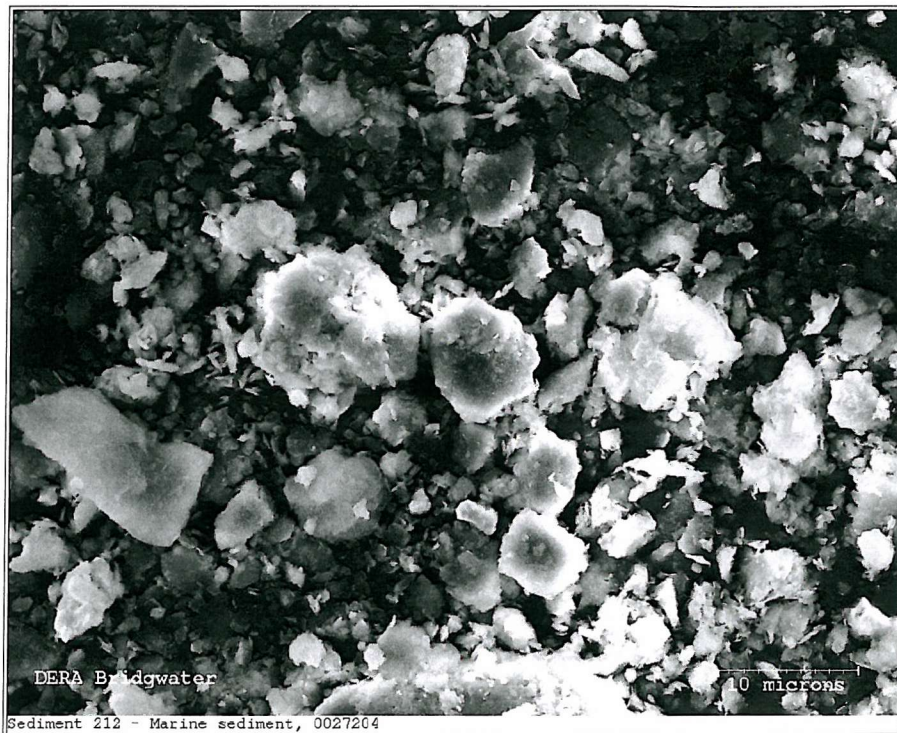
Figure 6.28. Scanning electron micrograph of sediment particles taken with an original instrument magnification of \times 2000 .
