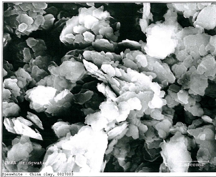
Figure 6.20. Scanning electron micrograph of Speswhite particles taken with an original instrument magnification of \times 10000 - another detail of area shown in Figure 6.18
