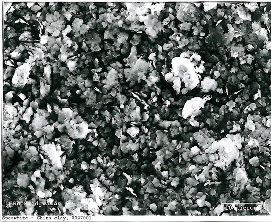
Figure 6.18. Scanning electron micrograph of Speswhite particles taken with an original instrument magnification of \times 2000 .
