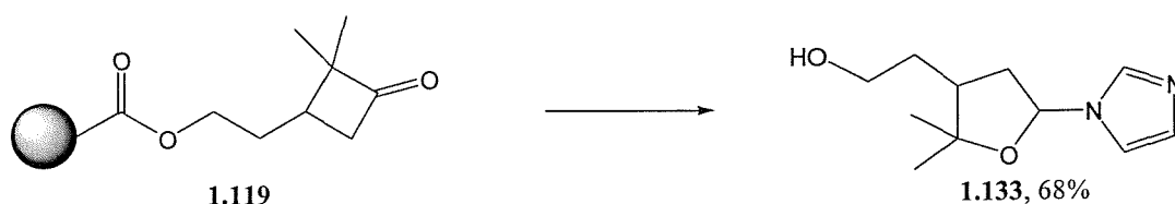
Scheme 1.43. Tandem ring expansion/addition of imidazole to cyclobutanone 1.119.
