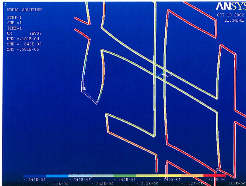
Figure 4.28: Static deflection of the two-dimensional meander actuator, displacement in x-direction is colour-mapped, dimensions see figure 4.27.
