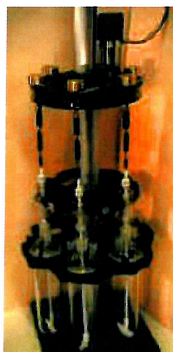
Figure 1. The reactor system. At the top right is the Brushless D.C. motor, beneath is the drive 'gearbox' system. Below is the set of drive shafts to the glass reactors in turn below. In the photograph only 3 reactors are mounted. Capacity is 6 reactors.
