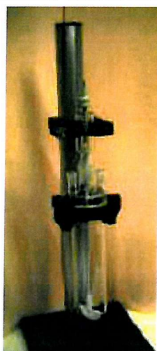
Figure 3. Reactor system held in the stand. The glass reactors, sealed and containing their stirrers (PTFE blade: 65mm diameter, stirrer: 500mm length from Aldrich) can be safely mounted and then filled or dismantled in the stand.
