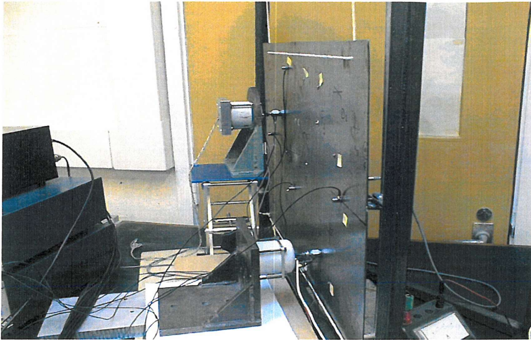
Figure 7.1. Experimental set-up for rectangular plate.
