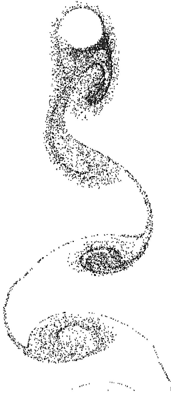
Figure 3.5: Wake patterns generated behind isolated rotating cylinder for R_e = 100 and angular rotation \gamma = 1.0
