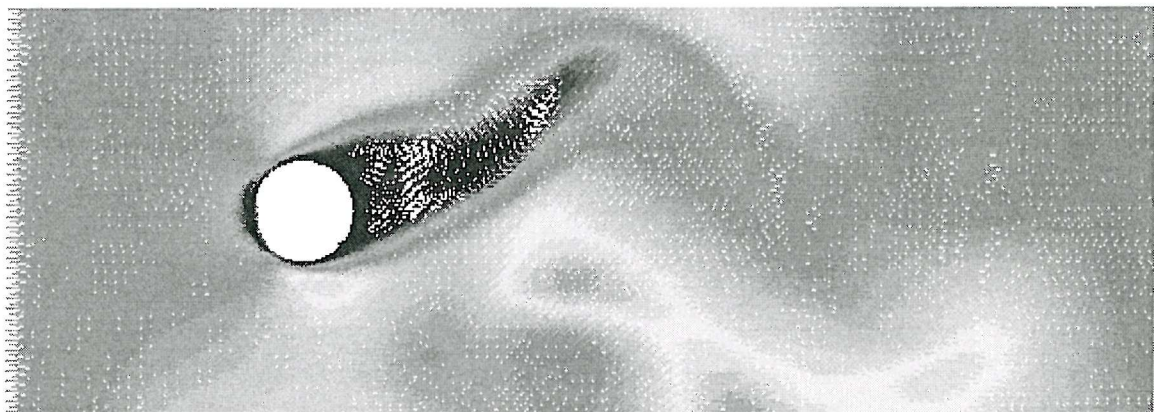
Figure 5.17: Velocity flow field at time t = t_0 + 6 seconds for Re = 100 with control in the time interval [t_0, t_0 + 6] seconds.
