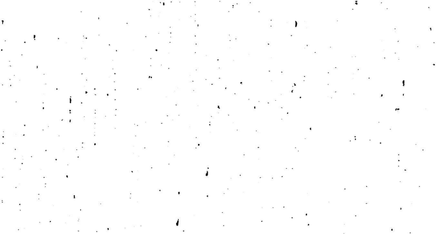
Figure 5.4: a) Optical micrograph of the L-S face of the 7150 W51 alloy, polished and unetched, b) Binary image of Fig. 5.4.a) showing the black particles and grey particles, c) Binary image of Fig. 5.4.a) showing the black particles.
