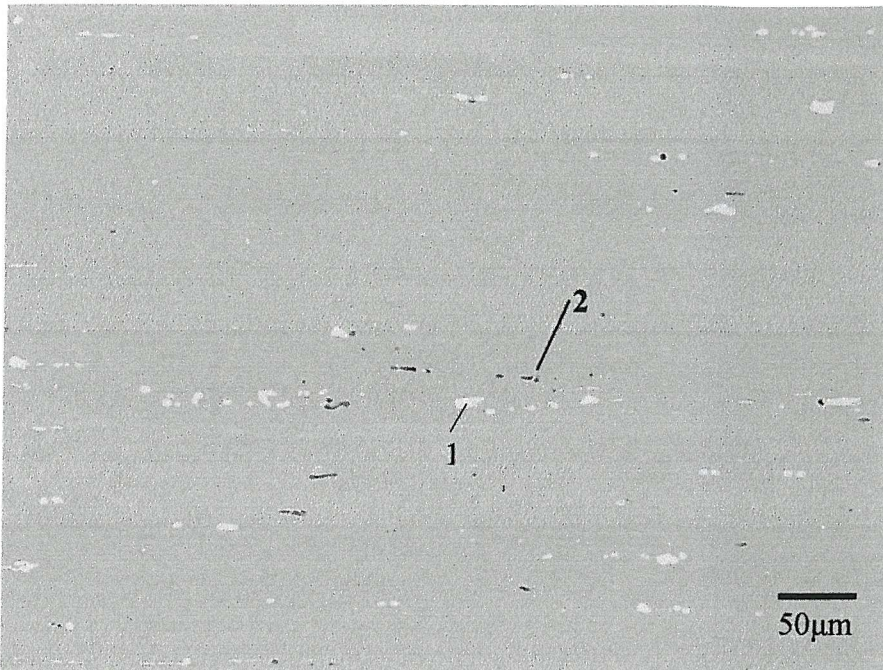
Figure 5.2: SEM backscattered image of LS polished section of the 7150W51 alloys where a systematic EDS analysis was performed on particles. Particle 1 was identified as 70%at Al-19.49%at Cu-9.43%at Fe-0.61%at Zn and particle 2 as 43%at Al-21.25%at Mg-34%at Si-0.5%at Cu-1.2%at Zn- Fe trace.
