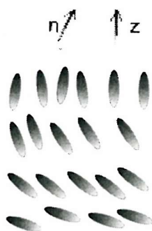
Figure 2.5 The chiral smectic C* phase showing the director \underline{n} precessing from layer to layer
