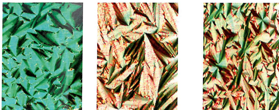
Figure 6.7 a) Smectic C* texture for no illumination at 60°C b) 286 mW/cm 2 at 60°C c) no illumination at 80°C.
