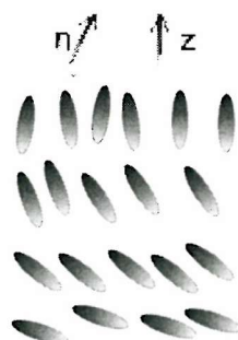
Figure 1.5 The chiral smectic C^* phase showing the director \underline{n} precessing around \underline{z} from layer to layer.
