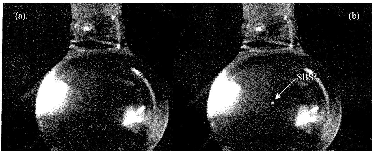
Figure 1.12 Frames showing the generation of single bubble sonoluminescence in a degassed water solution. The ultrasonic frequency was 27.744 kHz and the acoustic pressure amplitude was 140 kPa. Frame (a) shows the cell before generation of SBSL and frame (b) shows the luminescing bubble in the centre of the cell. The pictures were recorded using an image intensified CCD camera. The other light present on frames (a) and (b) is due to reflections from a lamp.
