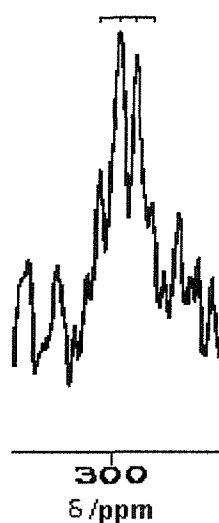
Fig. 3.7 The 89 Y NMR spectrum of [YBr 3 (Ph 2 MePO) 3 ] showing a quartet at \delta 299 ppm. The poor signal to noise ratio observed is due to the poor sensitivity of 89 Y and the modest solubility of the complex at 200 K.
