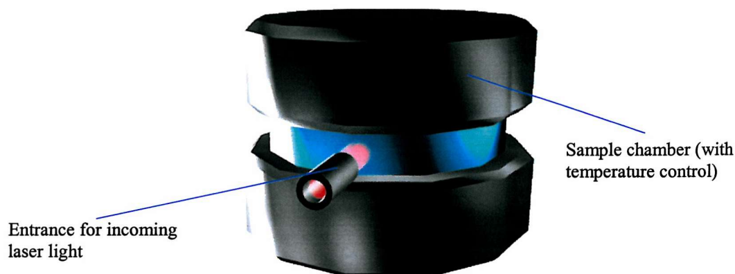
Figure 7.2: New sample holder.
