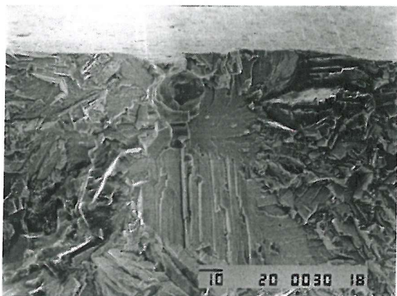
Figure 4-27a: U720Li-LG (Test 4S); primary crack initiation site (low mag).
