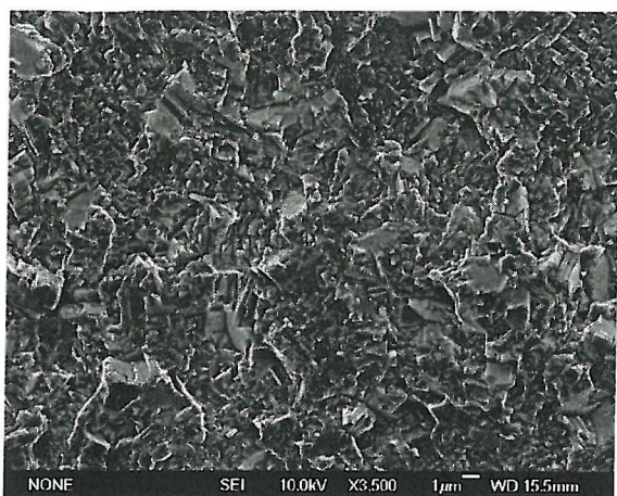
Figure 4-34g: U720Li-LP (Test 4T) Growth Out; ( \Delta K \approx 18.2 \text{ MPa}\sqrt{\text{m}} ).
