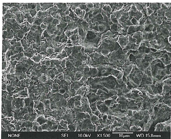
Figure 4-72a: RR1000; 725°C 1-20-1-1 Air ( \Delta K \approx 22.9 \text{ MPa}\sqrt{\text{m}} ).
