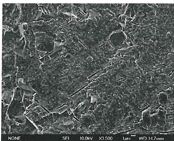
Figure 4-31i: RR1000 (Test 2T) Growth Out; ( \Delta K \approx 23.2 \text{ MPa}\sqrt{\text{m}} ).
