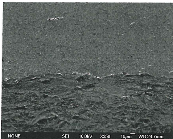
Figure 4-43i: U720Li-LG 840MPa Replica (Test 8HS); top surface of primary crack initiation site 350x.
