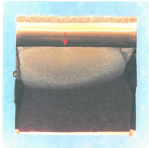
Figure 4-40b: U720Li 800MPa runout (Test 4HS); overall fracture surface.
