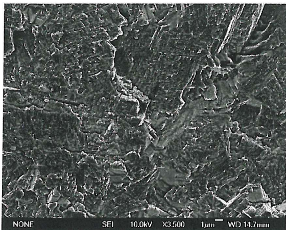
Figure 4-31g: RR1000 (Test 2T) Growth Out; ( \Delta K \approx 18.7 \text{ MPa}\sqrt{\text{m}} ).
