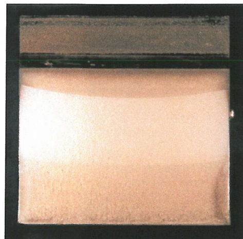
Figure 4-60d: RR1000; 725°C 1-1-1-1 vacuum (Test 5); overall fracture surface.
