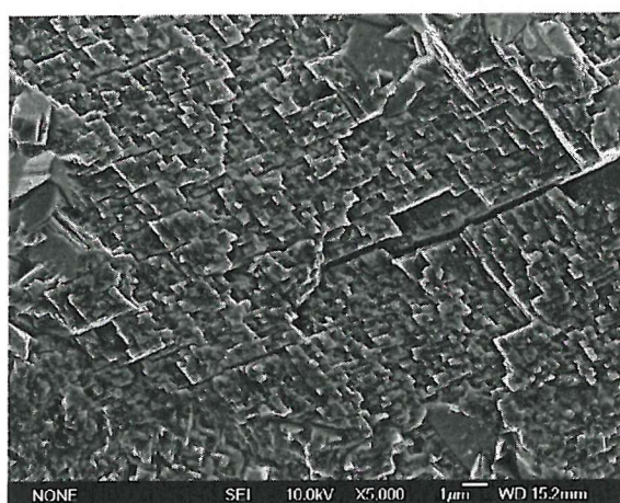
Figure 4-33e: U720Li-LG (Test 3T) Load Shedding; ( \Delta K \approx 14.4 \text{ MPa}\sqrt{\text{m}} ).
