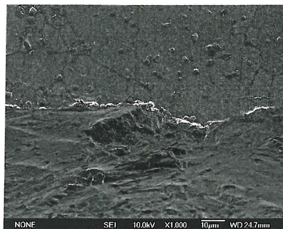
Figure 4-43j: U720Li-LG 840MPa Replica (Test 8HS); top surface of primary crack initiation site 1000x.
