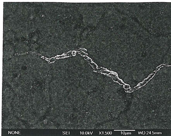
Figure 4-43h: U720Li-LG 840MPa Replica (Test 8HS); top surface of example secondary crack #2.
