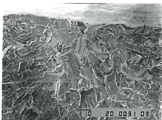
Figure 4-27e: U720Li-LG (Test 7S); initiation site at one of the secondary cracks.
