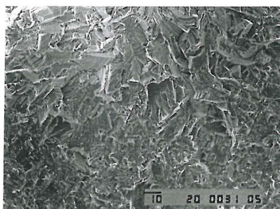
Figure 4-27f: U720Li-LG (Test 7S); Stage I to Stage II transition (approx. 0.10mm below surface).
