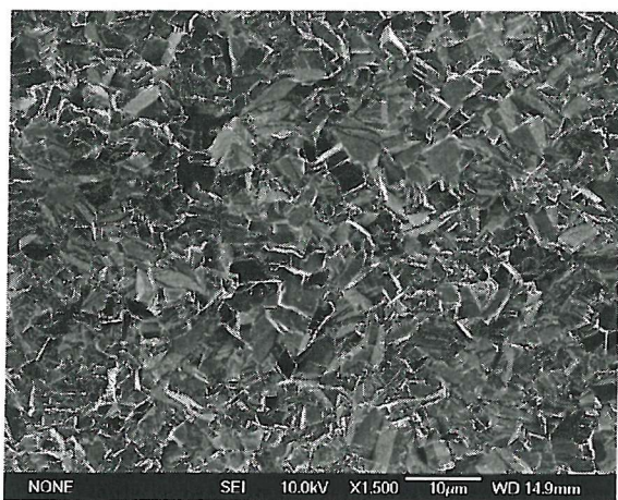
Figure 4-32a: U720Li (Test 1T) Load Shedding; Low Mag ( \Delta K \approx 7.5 \text{ MPa}\sqrt{\text{m}} ).
