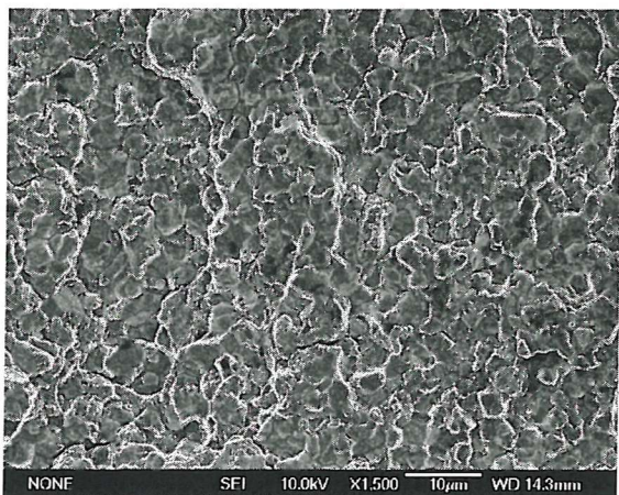
Figure 5-14a: U720Li; 650°C 1-1-1-1 Air ( \Delta K \approx 23.4 \text{ MPa}\sqrt{\text{m}} ).
