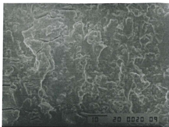
Figure 4-62b: RR1000; 650°C 1-20-1-1 vacuum ( \Delta K \approx 37 \text{ MPa}\sqrt{\text{m}} ).
