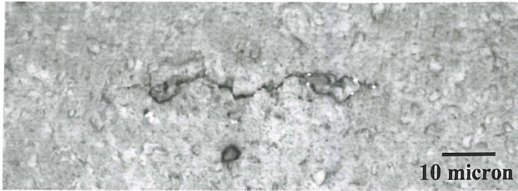
Figure 4-52a: Test 3HS - Crack 12, 13000 cycles 1000x
