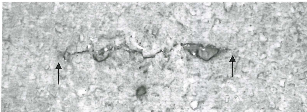
Figure 4-52d: Test 3HS - Crack 12, 16000 cycles 1000x
