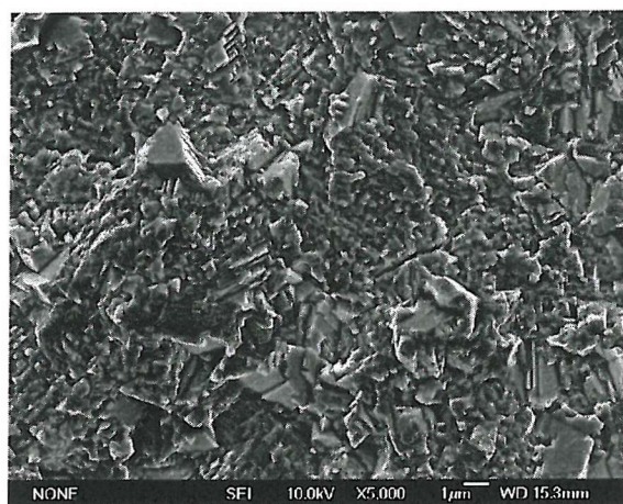
Figure 4-34e: U720Li-LP (Test 4T) Load Shedding; ( \Delta K \approx 14.5 \text{ MPa}\sqrt{\text{m}} ).
