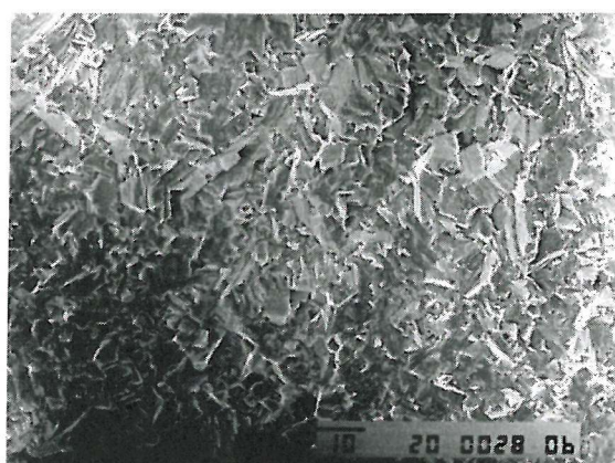
Figure 4-25d: RR1000 MO1751 (Test 3S); stage I to stage II transition (approx. 0.25mm below surface).
