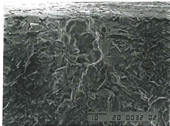
Figure 4-28b: U720Li-LP (Test 6S); primary crack initiation site (high mag).
