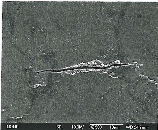
Figure 4-43g: U720Li-LG 840MPa Replica (Test 8HS); top surface of example secondary crack #1.
