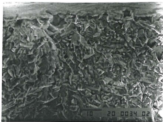
Figure 4-26b: U720Li (Test 10S); primary crack initiation site (high mag).
