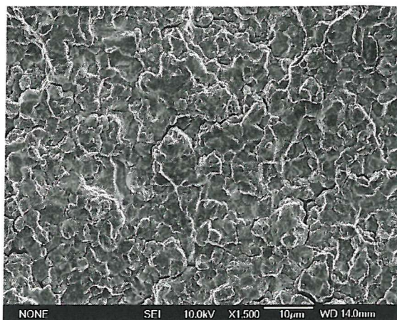
Figure 5-14b: U720Li; 650°C 1-1-1-1 Air ( \Delta K \approx 34.6 \text{ MPa}\sqrt{\text{m}} ).
