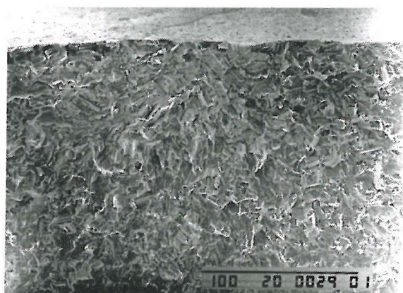
Figure 4-25e: RR1000 MO1547 (Test 8S); primary crack initiation site (low mag).
