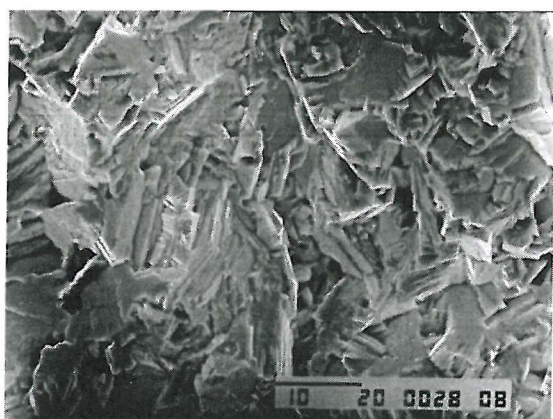
Figure 4-25c: RR1000 MO1751 (Test 3S); stage I crack growth (approx. 0.12mm below surface).
