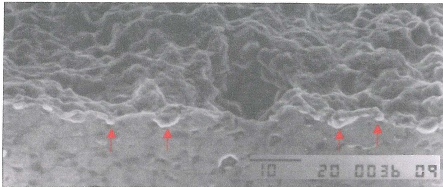
Figure 4-53: Test 3HS – Crack 12 top surface SEM.
