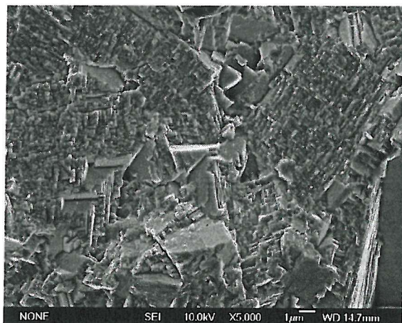
Figure 4-31e: RR1000 (Test 2T) Load Shedding; ( \Delta K \approx 13.7 \text{ MPa}\sqrt{\text{m}} ).
