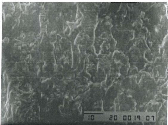
Figure 4-61a: RR1000; 650°C 1-1-1 vacuum ( \Delta K \approx 16 \text{ MPa}\sqrt{\text{m}} ).
