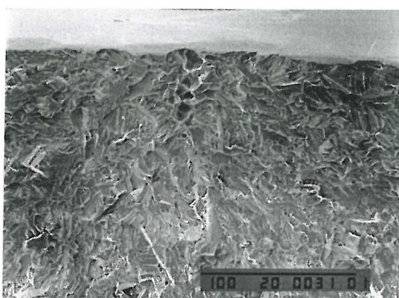
Figure 4-27c: U720Li-LG (Test 7S); primary crack initiation site (low mag).
