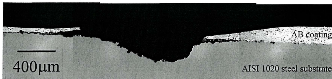
Figure 6-7 Optical micrograph showing an area of the transverse section where the coating was penetrated after 5 days of erosion-corrosion. 3.0 \text{ ms}^{-1} , 20^\circ\text{C} , 3.5 % NaCl, 5 % w/w sand concentration.
