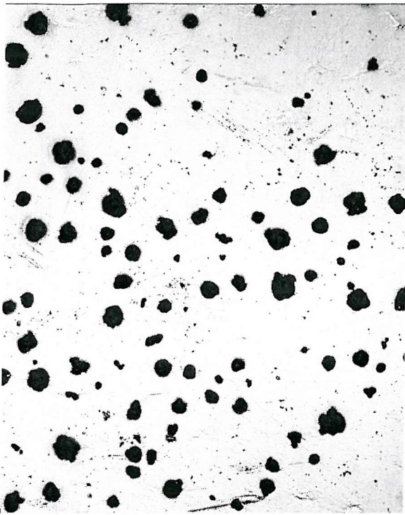
Figure 5.5: Image of a '900/390' specimen for use in graphite nodule distribution analysis.
