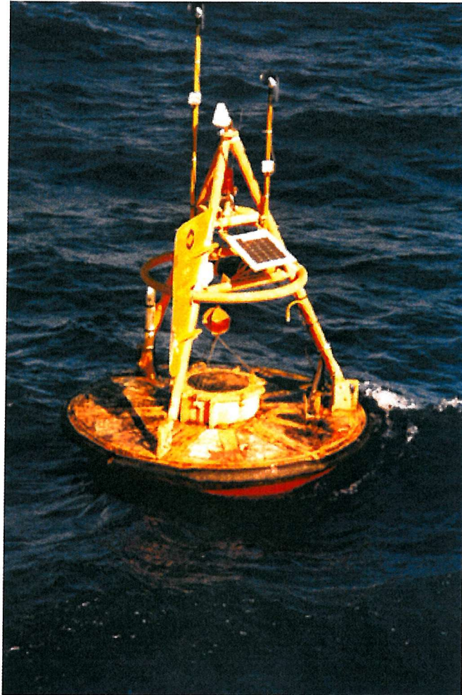
Figure 2.2: Heave-pitch-roll buoy in operation in Campos Basin. The hull has a diameter of 3 m, the structure has a height of 6 m with a total weight of 1500 kg.
