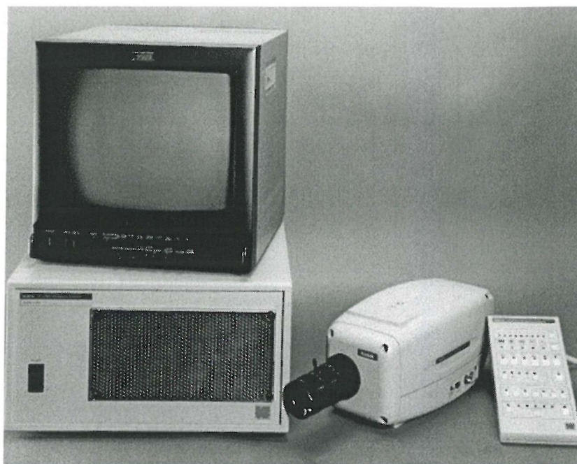
Figure 2.10 A photograph of the Kodak HS 4540 high-speed video camera used to record images of an oscillating bubble.
