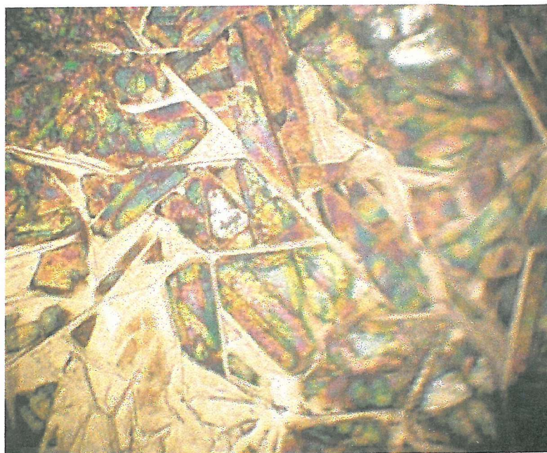
Figure 5.10. Light microscopy of a freshly washed mesoporous nickel electrode film shows a surface divided into domains.
