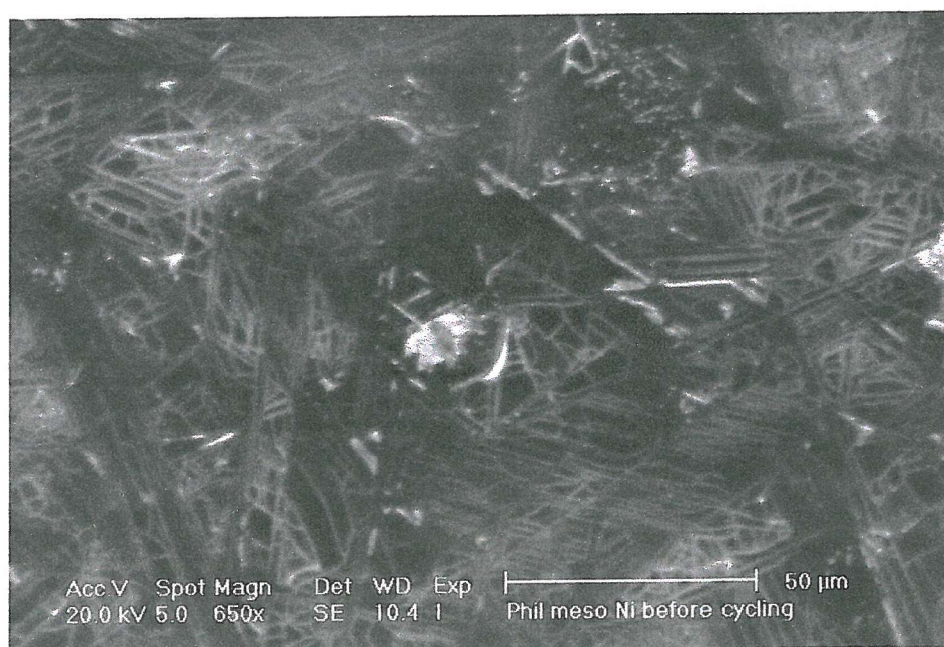
Figure 5.11. Contrast in this SEM image shows the domain boundaries of a freshly washed H 1 mesoporous nickel film. The structure is very similar to that observed in Figure 5.10.
