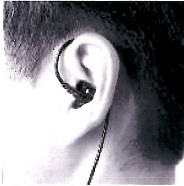
Figure 3.10: Example of a body-conduction microphone placed in the ear-canal of the user.
