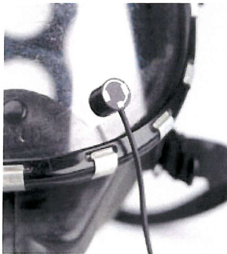
Figure 3.9: Example of a mask microphone used for underwater and firefighters' communication.
