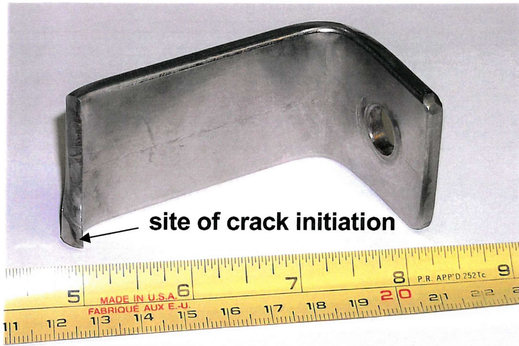
fig.4.7 Cracked Spacer Bracket
